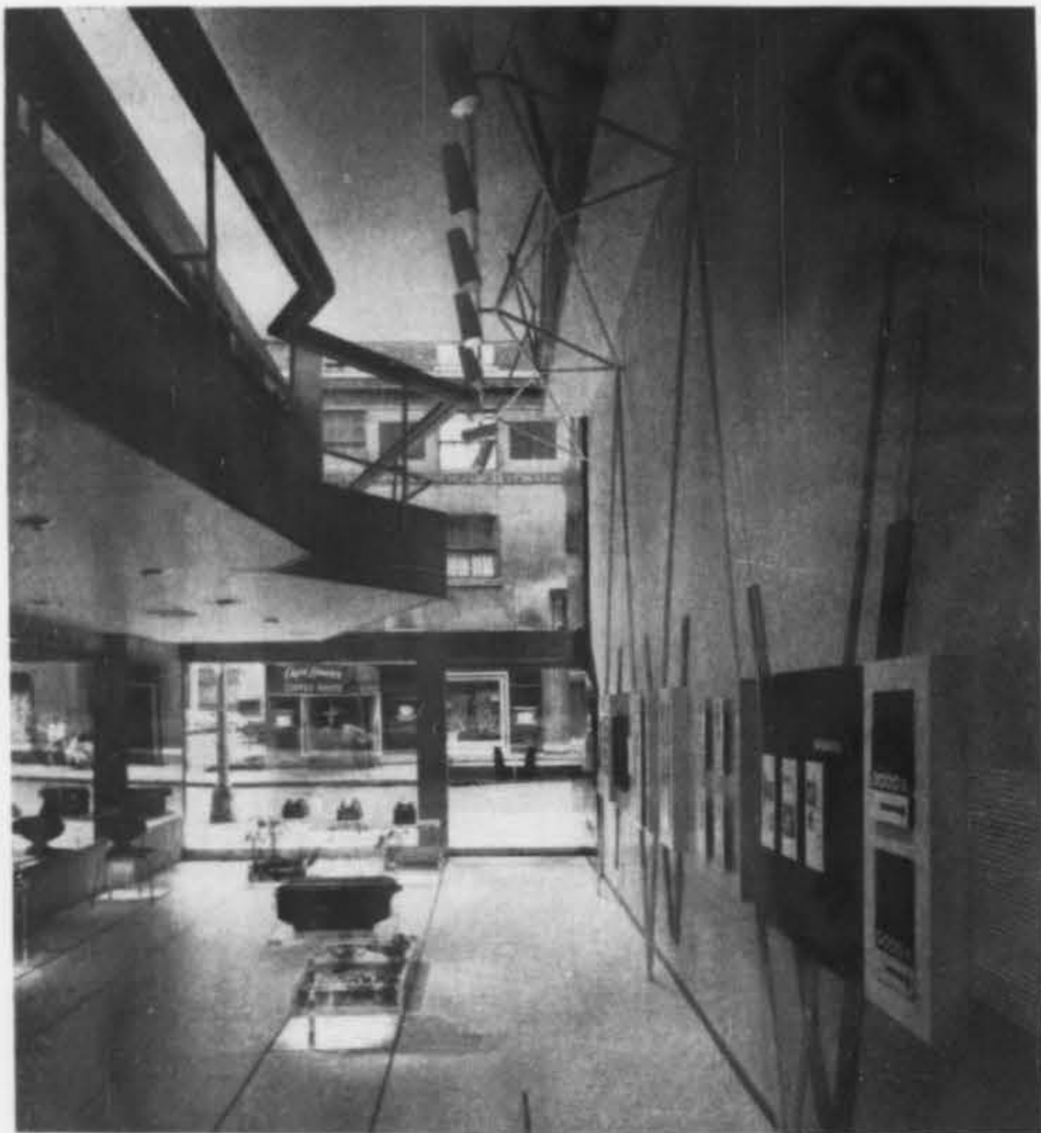
View to front. Rail parallels balcony, pipework unites lights and display wall.
