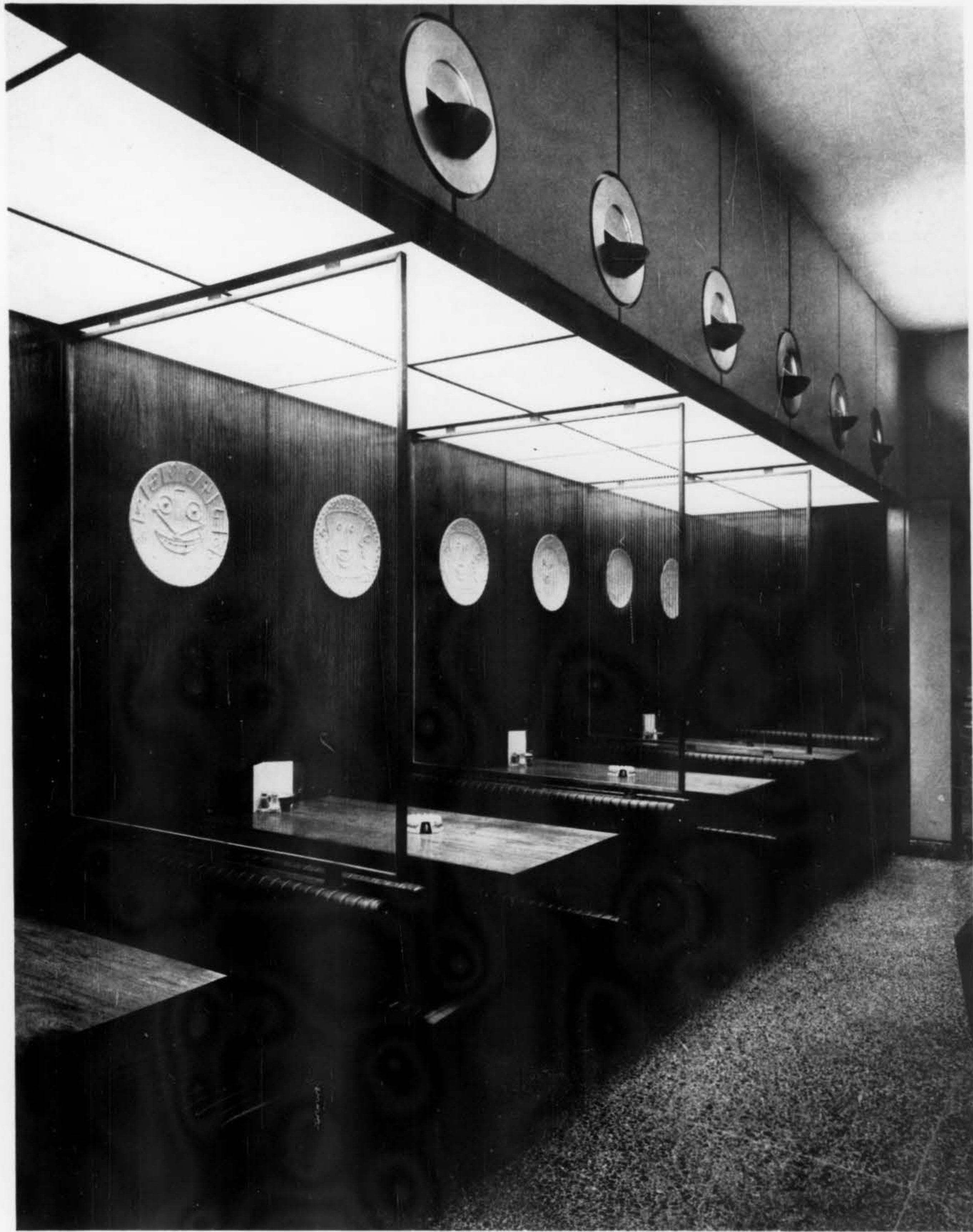
Series of recessed booths that surround counter area are afforded a sense of privacy by dividers of striped glass (Pittsburgh Plate). Ceramic plates by Picasso are mounted on teak panels (all woodwork by Langenbacher). Floor is terrazzo (Sidney Foscato).
