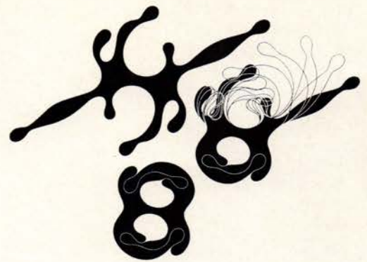
5. NEGATIVE/POSITIVE EXTRUSION —A molding which closes in upon itself to form channels acts as a lamp housing. The advantage of a flexing, sealed raceway which allows access to wires and functions as a fitting for fixtures is economically realized in this design.
