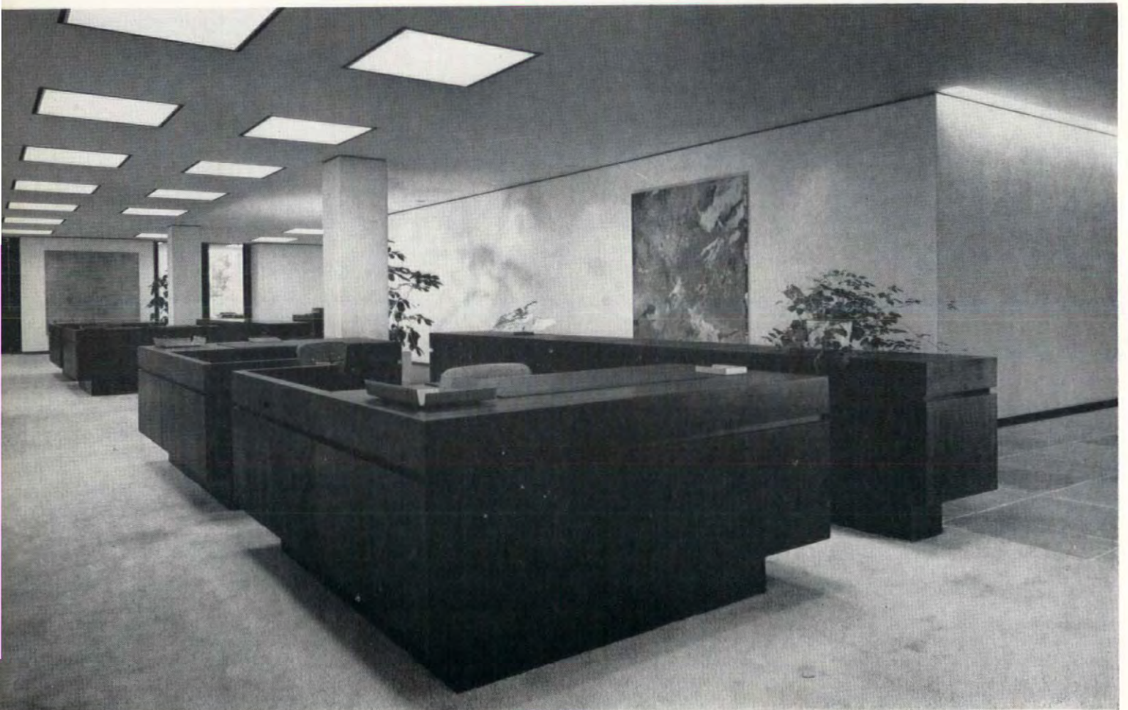
Above: Secretarial stations formed by massive wood desks and credenzas lacquered in dark cordovan finish create the traffic pattern. Walls are natural plaster in sand-textured aggregate in harmonious contrast with beige carpet and bluestone floors. Lighting fixtures incorporate air conditioning vents.
