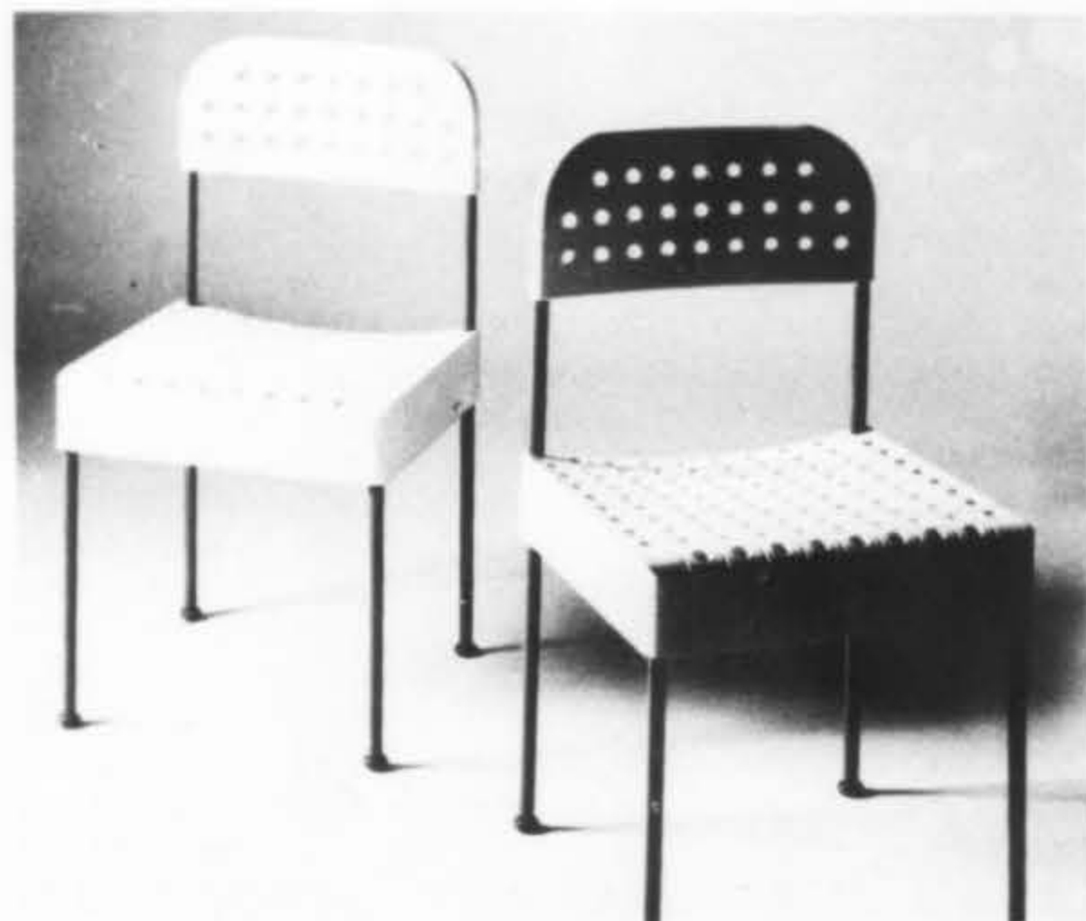
Castelli The new KD "Box" chair (above), designed by Enzo Mari, packs into a to-table package. Six pipes insert into seat and back. Colors of perforated, molded polypropylene seat and back are white, green, yellow, or brown. Frame is metal covered by a sleeve of PVC. New to U.S., chair has been used in a number of Italian restaurants. circle 259
