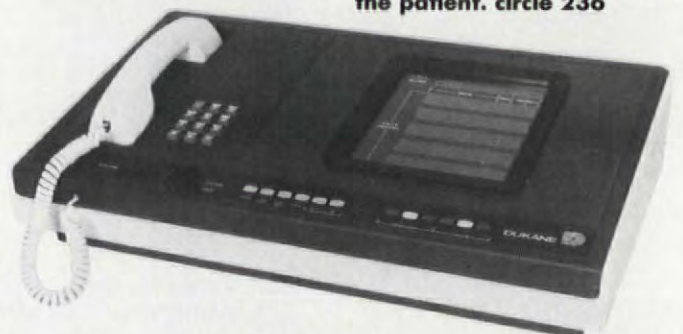
Above: The Dukane System 2070 Multiplex Communications System is a microprocessor-controlled hospital communications system capable of servicing 3072 beds. circle 237
