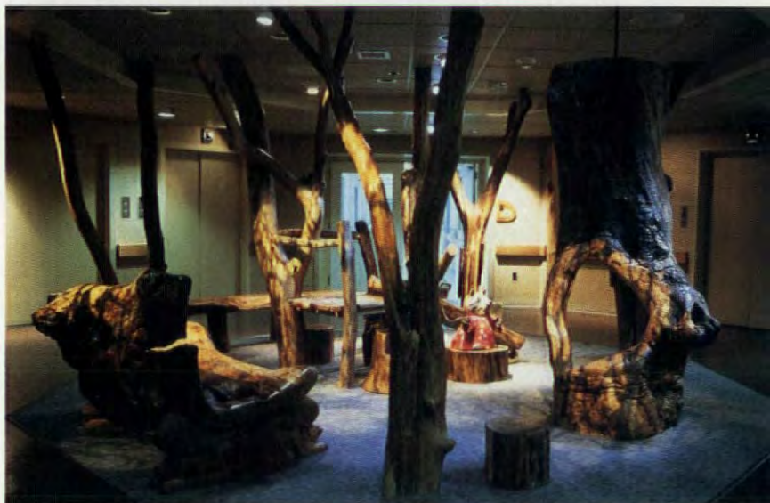
Above: The sculpture of trees is illuminated by a ceiling-mounted halogen lighting system with lens templates that simulate the dappled effect of light in a forest.
