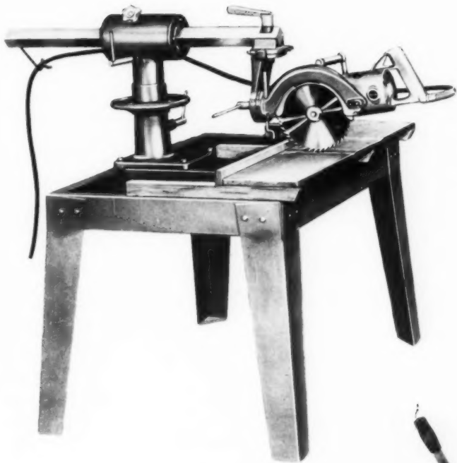
Professional Skilsaw can be hung on a radial arm to make a cut-off saw.
