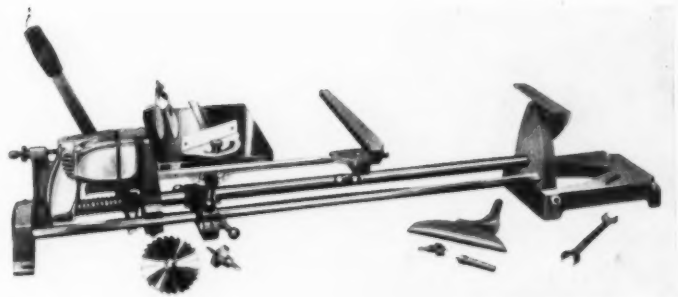
Cummins Do-It Shop, a combination unit powered by portable drill, appeals to amateurs intimidated by larger tools.
