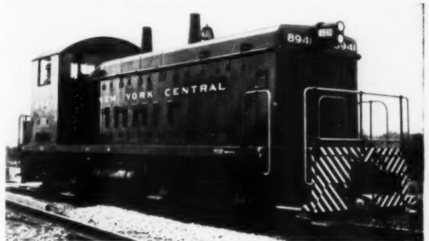
Standard switching locomotive "decorated" by safety markings.
