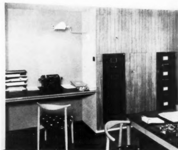
An office using Bartrev board on virtually all surfaces—walls, cabinets, tables, ceilings, shelves—is possible because the board's low cost permits a variety of colors and textures to be applied as veneers and finishes.
