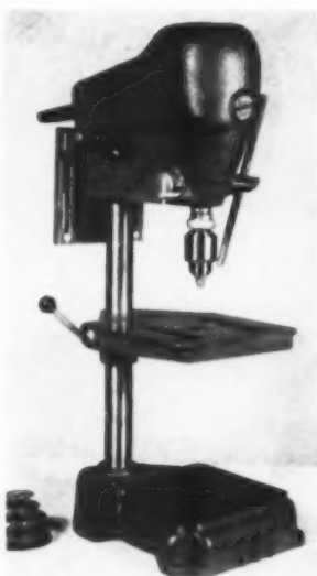
Hood shields pulleys of Delta drill press, left, envelopes mechanism of streamlined Darra James.
