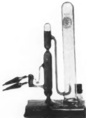
All-glass model of heat-powered Thermo-Pump, operated by electric or flame heat.
