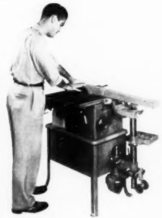
Delta's combination unit consists of separate tools mounted around one motor.
