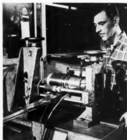
Precision slitting equipment for cutting rolled strips to width.
