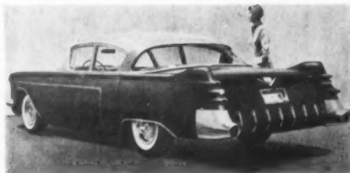
Panoramic back window does away with blind spot, but as experimental Cadillac shows, front and back windows are enlarged at expense of view outside.
