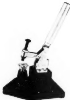
Press for assembling tube sockets on wafer (above) and (below) assembly fixture for holding wafers while wires are soldered into notches to complete module.
