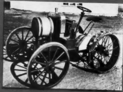
Automotive beginnings of the modern tractor: Henry Ford's 1907 experiment with an "automobile plow" had 24 h.p. engine, rear wheels taken from farm binder.
