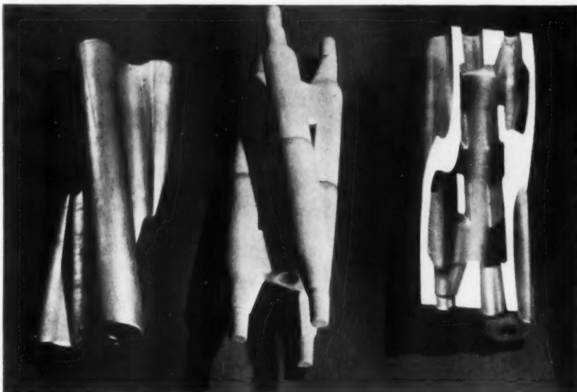
(Center) Sand core for aluminum casting made with Bakelite resin. (Left and right) The finished casting is shown cut open to reveal cleanness of casting interior.
