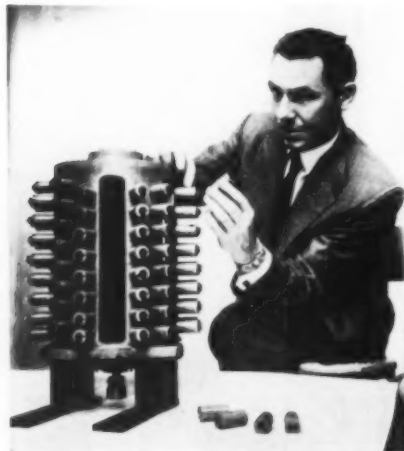
↑ Logistics Research, Inc. has unveiled the ALWAC, a new all-purpose electronic digital computer whose low cost ($48,000) may bring it into commercial use. The rotating magnetic memory drum stores 2048 words; Logistics president Glen E. Hagen holds one of the heads which both "write" and "read."
