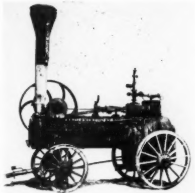
J. I. Case's steam engine No. 1 (1869) was pulled into the field by horses, supplied belt power for threshing and sawing.
