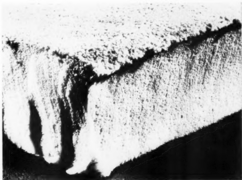
Plastic foam made from a plastisol based on a Bakelite vinyl resin.
