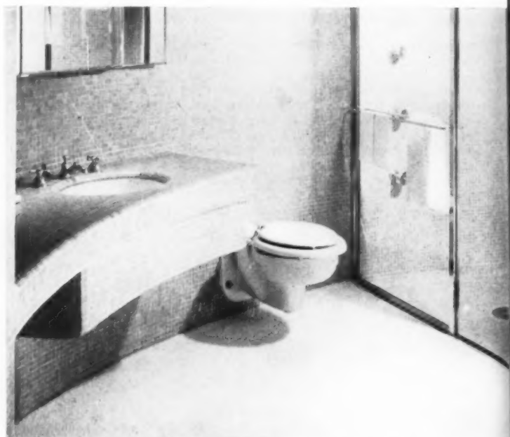
William Zeckendorf's private bath, the spiraling climax of a circular office, contains two ideals of modern bathroom design—the countertop lavatory and the wall-hung closet. Both have practical drawbacks.
