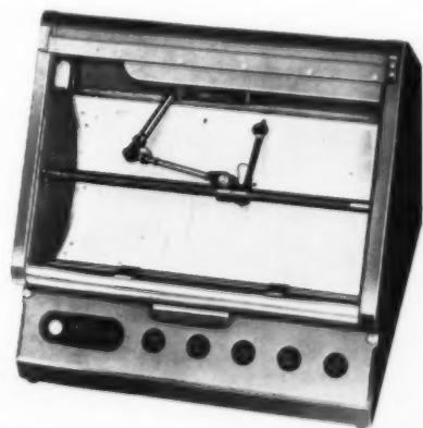
Librascope plotter makes a continuous graph of the relation between two factors.
