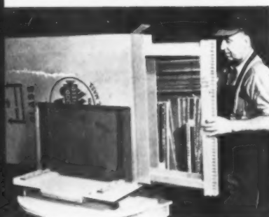
Shock-absorbent honeycomb replaces complex old packing for mirrors.
