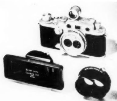
Leica's answer to 3-D is a twin-lens attachment
