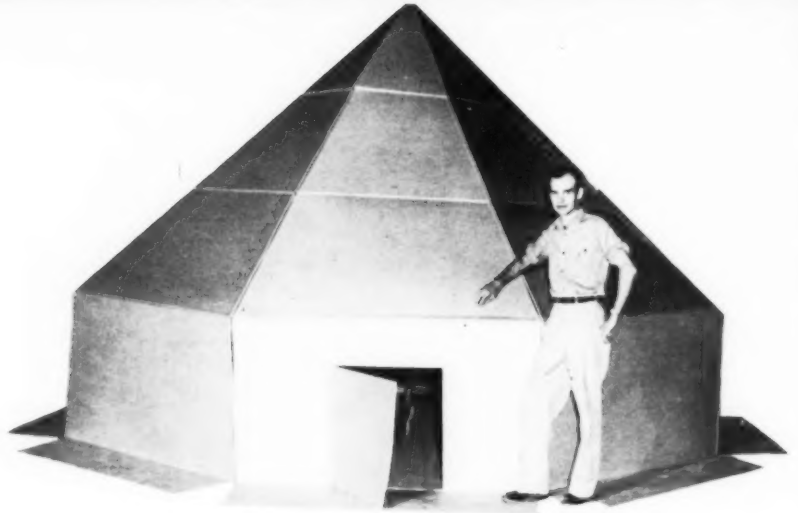
Gaylord 10-man tent comes in 8 flat sections joined on the site with a hand stapler. Board is highly sized and paraffined for water-resistance; seams may be caulked. Quartermaster tests indicate excellent heat retaining properties.
