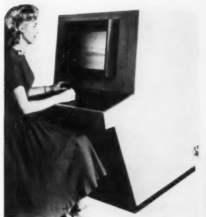
recorded on punched tape, punched card, or magnetic tape for use in digital computers; or fed to an electroplotter for final plotting. The sleek housing emphasizes simplicity and legibility. The Boscar, or ballistic film analyzer and recorder (right), a flying spot aligned with fingertip control, measures X-Y displacement.
