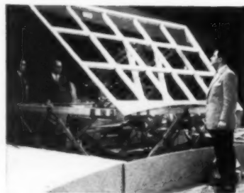
Tilt elevator lifts and tilts heavy displays.
