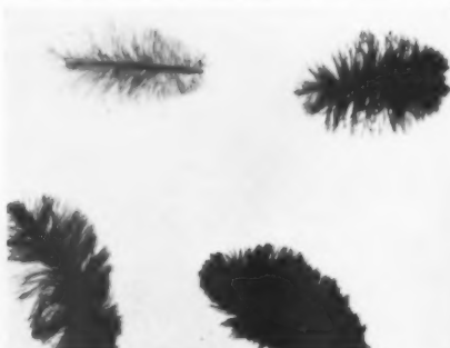
Polyplastex laminates of textile fibers (above) and bird feathers (below) in translucent sheet.
