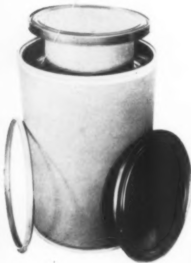
Continental Can's Payoffpak for wire is designed as a 3-in-1 labor saver: a fiber winding drum for wire off the drawing machine, a shipping carton and later a dispenser.
