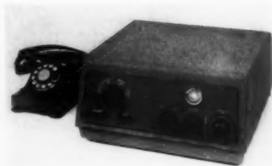
↑Bell Telephone Laboratories and designer Henry Dreyfuss collaborated on development of the Answering Set. Before going out, you tape a request that callers leave message. It plays when the phone rings, while another tape records the message; calls are all taped up when you get home.
