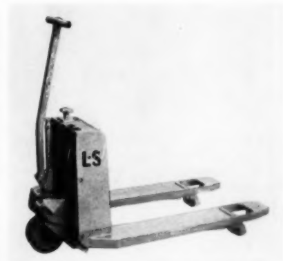
↑Lewis-Shepard heavy duty hand pallet truck, made of Frontier Aluminum alloy castings, weighs only 250 pounds but lifts two tons. Load is raised hydraulically by foot-operated lever. $447.50.
