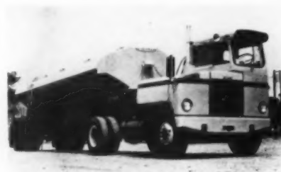
†Kenworth Motor Truck Corporation's new heavy-duty highway tractor was redesigned by Gideon Kramer. The one-man cab-beside-engine, large side windows, and the outboard mirror, increase the driver's visibility. All-aluminum welded construction makes it lighter than usual trucks.
