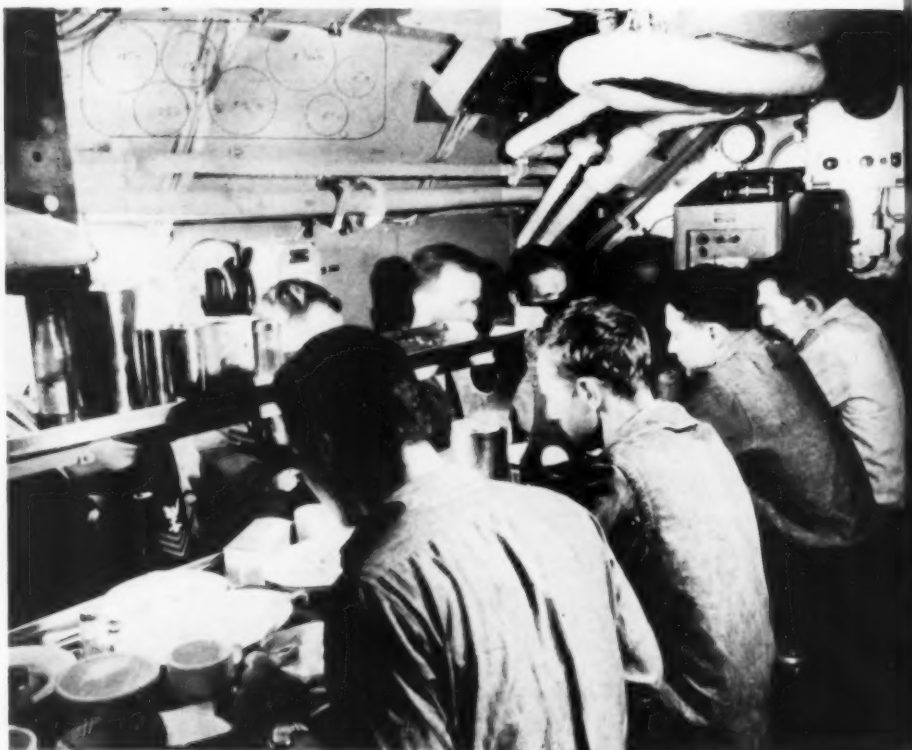
The crew mess area on a Trigger-class sub, above, graphically points up improvements on the Nautilus (opposite). Men are crowded together amid instruments and an overhead clutter of pipes and wiring. The laden shelf at eye level is a condiment tray. Its underside provides light for the table, since overhead suspended lights are virtually impossible, but the tray remains a permanent obstacle to vision and conversation.
