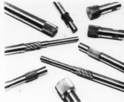
A variety of splined parts produced by the Roto-Flo process.
