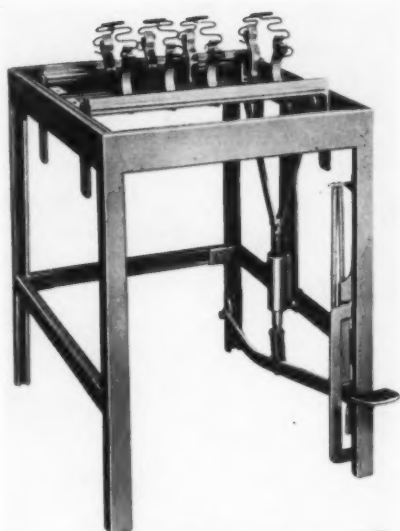
Automatic device for stretching and positioning No-Sag springs for attachment to chair frames.
