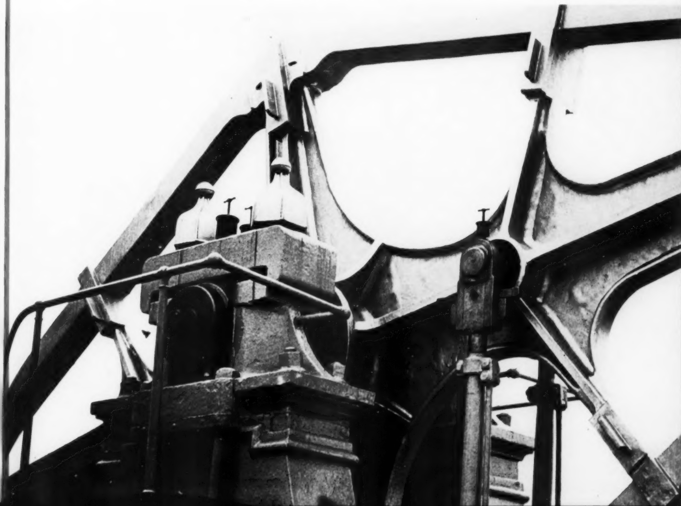
Part of the beam and its support, showing ornamental housings over the huge nuts that hold the frame together. 2
