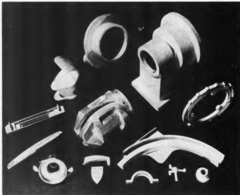
A group of aluminum castings made by the Alcoa plaster process. The trademark shield is 2 inches in height.
