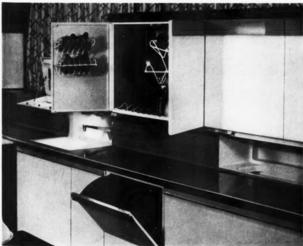
Dishes are washed, dried, and stored in wall-mounted unit. Incinerator is below, laundering machines are at right under counter. The sink, only non-GE item, could be integrally molded with plastic countertop.
