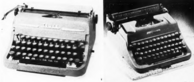
Tower portable typewriter was redesigned in 1953 by staff designers. Standard model, left, became a deluxe model with a full-length tabulator. Along with mechanical improvements, an embossed metal nameplate replaced the die-cut one, the housing was given a crisper shape, the fine wrinkle finish changed from blue-green to gray. Lettering and layout of the paper table was improved, new finger-shaped keys added.
