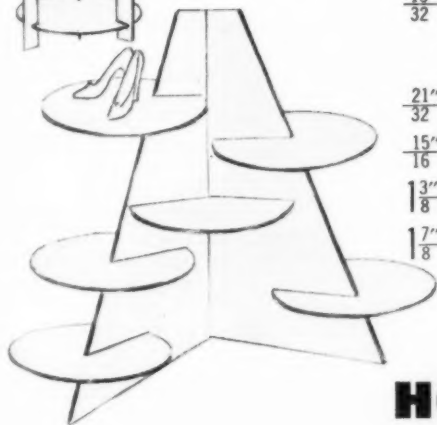
DISPLAYS designed by Tom Lee, Limited — slotted circles of Homasote Type RD fitting into other slotted members
