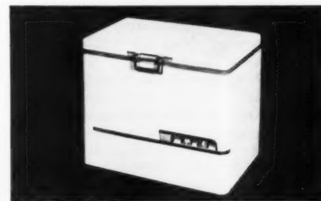
1953 model had a new compressor unit which enabled designers to eliminate front air grill. Low controls were used so that connections would not have to pass through insulation, thus preventing possible leaks where frosting could occur.
