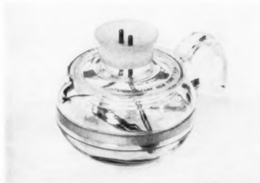
77 Ohmlette The Chemex Corporation, New York Dr. Peter Schlumbohm, inventor Tempered Pyrex bowl (Corning Glass) and lid; electrodes molded into nylon (Driver-Harris). Stainless steel coil heats quart of water in 5 minutes; if water evaporates, coil melts like a fuse.
