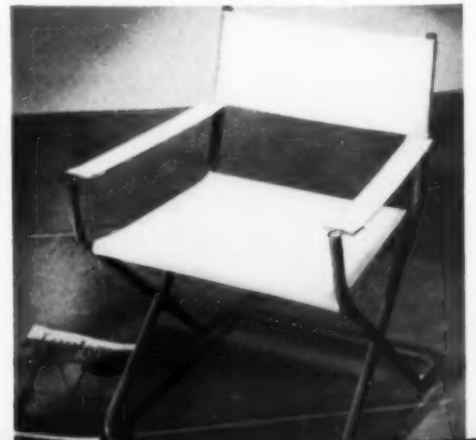
39 Catalina folding chair Hemet Sales Co., Los Angeles Merendino-Greene, designers Anodized aluminum frame (American Pipe & Steel); duck fabric. Weighs 3½ pounds.
