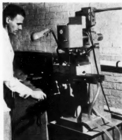
Ultrasonic machine tool. The tapering conical section vibrates against the material to be cut 25,000 times per second.
