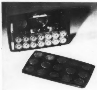
Miniature personal radio using transistor circuits and oscillator speakers.
