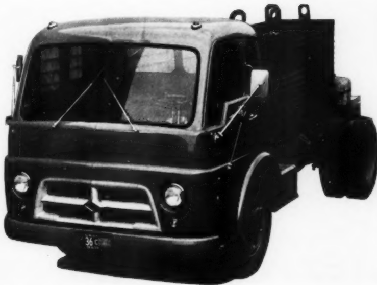
26 Cab-over-engine truck Diamond T Motor Car Co., Chicago Jan W. Hauser, consultant designer Stamped sheet metal body (McLaughlin Body Co.); die-cast aluminum grille (Acme Aluminum); Solex glass (Pittsburgh Plate Glass).
