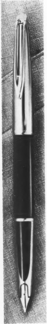
34 C/F Fountain pen Waterman Pen Company, Seymour, Conn. Harley Earl, Inc., consultant designers Injection molded acrylic barrel (Bakelite); 14 K gold nib (Handy & Harman); gold- plated brass cap, Teflon-coated spring in- sert; polyethylene cartridge, heat-sealed after filling.
