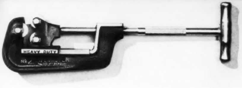
24 Pipemaster pipe cutter Erie Tool Works, Erie, Pa. Wilbur Henry Adams, consultant designer Shaft and handle of formed steel, welded together inside; shaft red. Spring steel pin permits rapid change of size.
