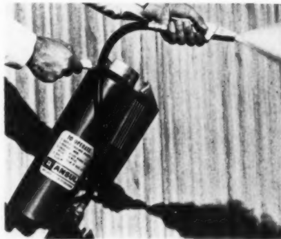
↑ Ansul's newest fire extinguisher designed by Raymond Loewy Associates weighs 22 pounds, and expels 10 pounds of dry chemicals. Bonderized drawn steel shell with red baked enamel finish, cadmium-plated brass hose couplings. $52.50.
