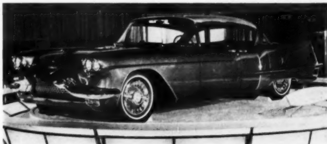
Cadillac Eldorado Brougham has hooded headlights, shark-fin bumpers, duck-under grille, individual seats for four passengers. Front seats pivot for easy ingress. Metallic green with complementary interiors. →
