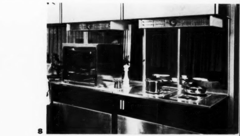
8 Cooking center's recessed hotplates flip over when not in use; underside of one is a griddle. Oven rises from counter and, like drop-down controls, works from kitchen or patio.
