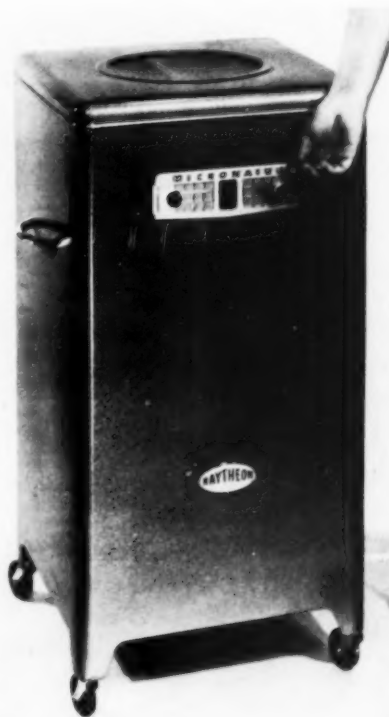
↑ Raytheon "Micronaire" room air cleaner is an electrostatic precipitator with cell and ionizer assemblies that can be removed as a unit for washing. Weighing 60 pounds, it is 15" square, 30" high. Designed by Leonard Emerson. $229.
