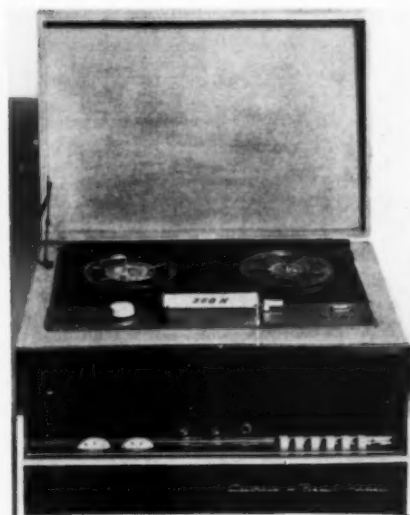
↑ Columbia-Bell & Howell 360K (for Kilo-sphere speakers) has a plywood case and a front grille with controls on a step so that the recorder can be operated with lid closed. Push button control of reels and thumb dials for volume and tone control simplify and speed up operation. Two pulse lights indicate normal recording level and peaks.
