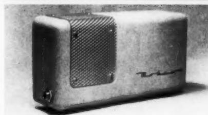
↑ Mohawk Midgetape has a spotwelded sheet aluminum case and operates on hearing aid batteries with a life of 45 hours. External power amplifier has a 2" speaker, with anodized aluminum cover on a drawn steel case. Light grey wrinkle finish with silkscreen red lettering on both. Designed by Fred Bohm.
