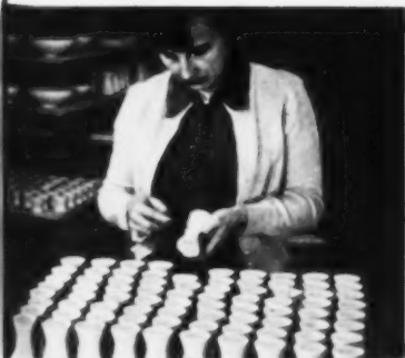
Trude scrapes mold marks from dry pieces, now white. Harold dips each piece in glaze for final finish before putting it in kiln where heat fuses clay into hard white porcelain. Firing cycle takes one day to heat slowly, two more to cool off again.
