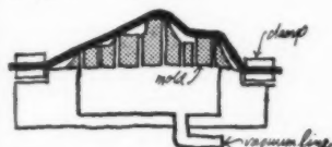
Framed sheet is stretched over male plug before vacuum is pulled
