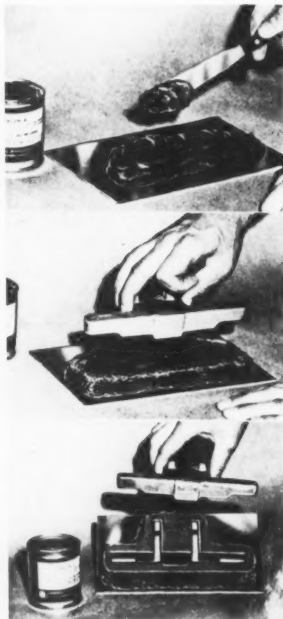
Devcon being used like putty. After hardening agent is added, it becomes a steel-like mass.
