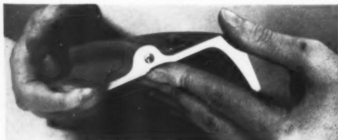
Sample casting shows enameling of inserts, irregular planes.
