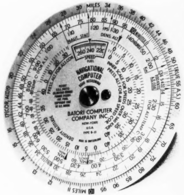
Navigation computer markings are applied photographically.
