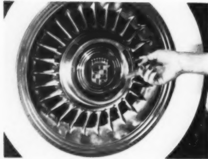
† Cadillac Eldorado wheel is forged bright-chrome-plated aluminum.
