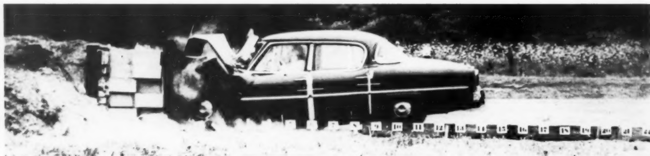
Doors stay closed as test car with new safety latches crashes head-on into barrier.
