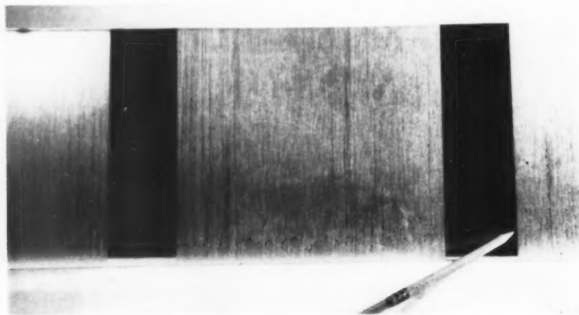
Comparative reflection and absorption of light striking various aluminum surfaces that have been polished and given a standard anodic coating of about five microns.
