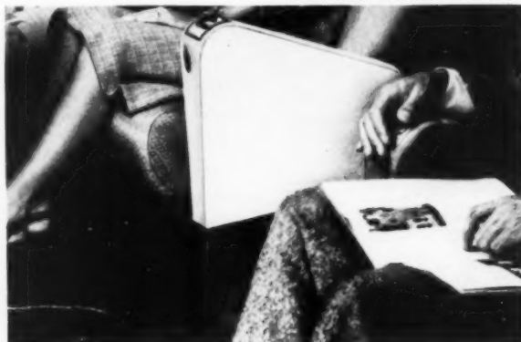
SCUFF PLATES throughout the plane use a silver sheet of durable metalized "Mylar"; this new material will not tarnish or embrittle.
