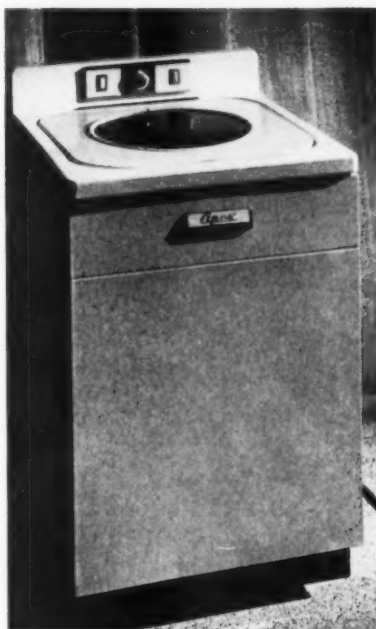
19 Kitchen-Aid dishwasher Hobart Mfg. Co., Troy, Ohio Steel tank, porcelain-enameled, stainless steel fittings; formed steel support frame; cabinet panels in baked synthetic enamel finish; plastisol-coated steel baskets.
