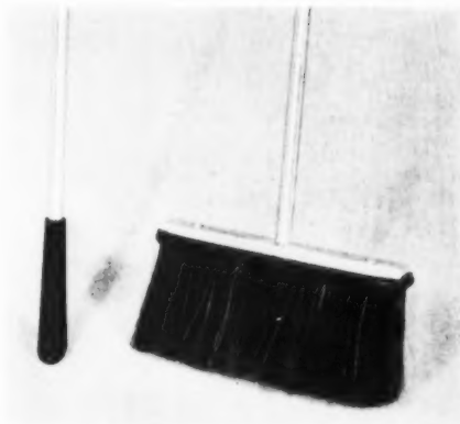
30 Slim-line broom Stanley Home Products, Inc., Easthampton, Mass. Steel back (Elliott Bros.), welded tube (Van Huffell); bright zinc finish; molded rubber bumper (Acushnet); twin-faced strip brush.
