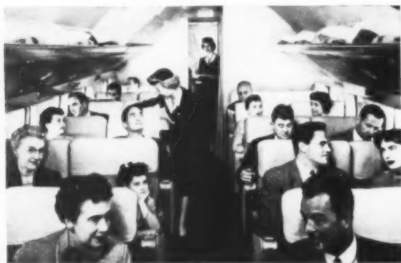
BULKHEAD PANELS employ a sheet of gold "Mylar" laminated to rigid backing, which lends striking depth and sheen to cabin area.
