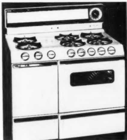
22 Kaiser gas range Coburn Stove Co., Tapton, Pa. Peter Muller-Munk, consultant designer Stamped steel body, porcelain enameled white or five colors; molded urea knobs (Fational Lock), white with chrome trim; stainless steel rolled sections on backguard (Pyramint Moulding), die-cast end caps (Stalle Corp.); ceramic insert in glass (Chromone Co.)
