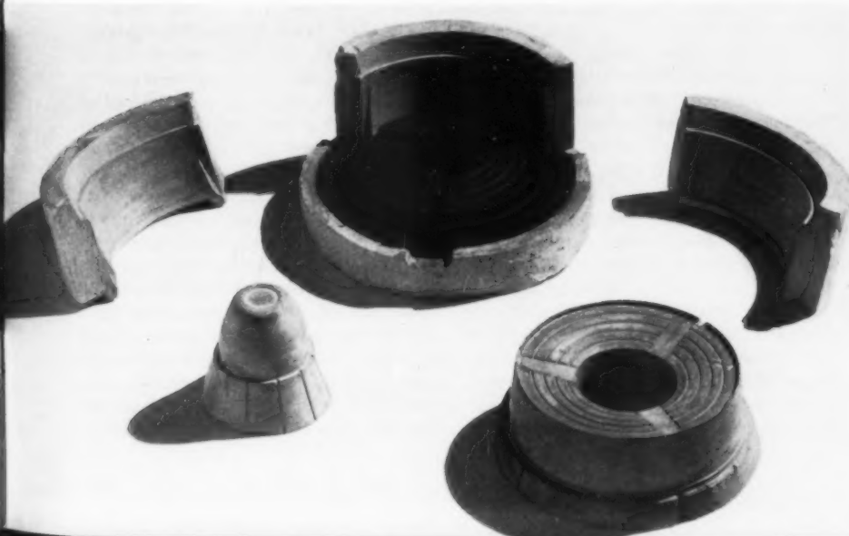
6. Cores, piece mold and flexible mold are disassembled and prepared for casting. The original plaster model is removed, creating a cavity into which, after reassembly of the mold, the epoxy casting resin is poured.
