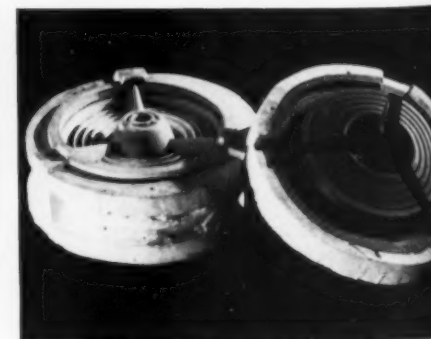
5. The cap piece is again taken off. The elastomer mold is removed from the model and placed in the cap piece.
