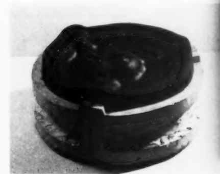
3. A thickness of clay is placed over the grill portion of the model and the top edge of the piece mold.
