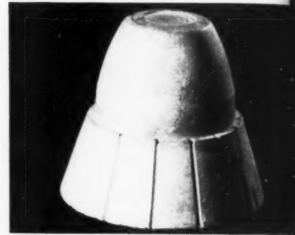
1. Initially, a core for the fan motor housing is turned in plaster with the aid of zinc templates.
