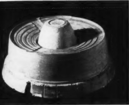
2. A core for the fan heater housing and front grill are similarly turned in plaster and related to the fan motor housing core. Then an original plaster model is turned and fabricated over the cores,
