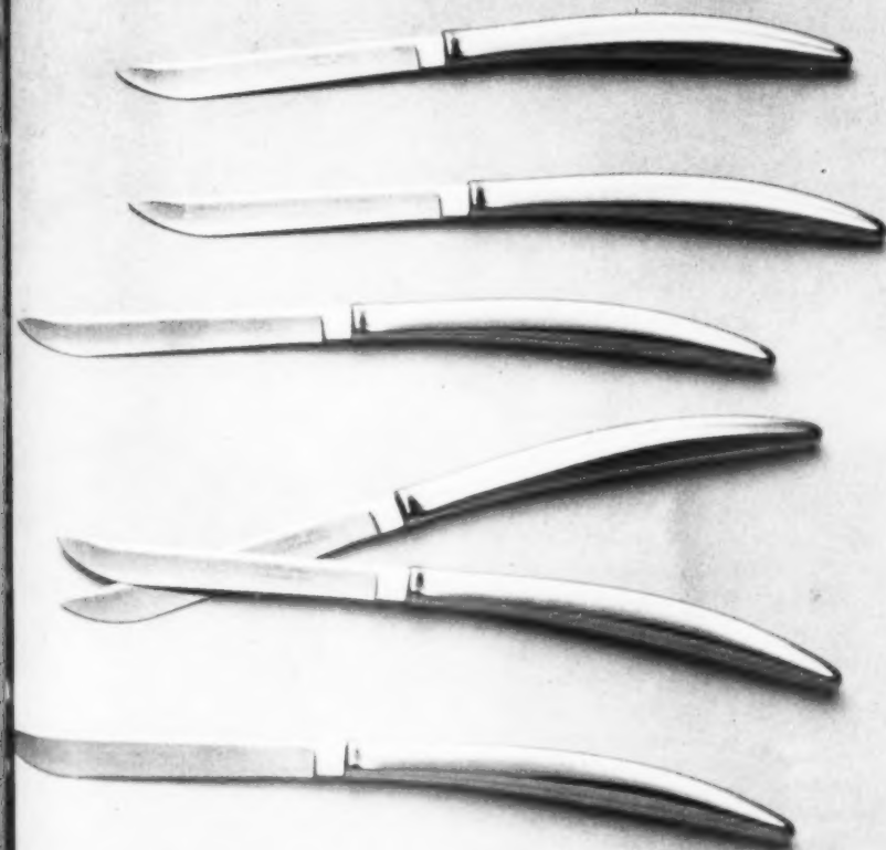
Companion steak knife set has a chrome-plated cast-zinc handle pressure-fitted to stainless blades.
