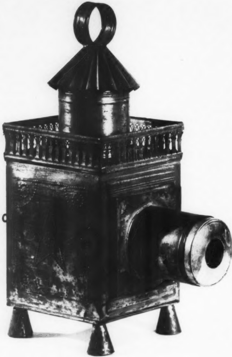
Projection lantern of late 18th century; light source—a single candle.
