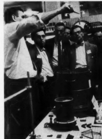
Polymer Whirlclad coating process. A heated object is dipped into powdered plastic which is fluidized by an ascending current of air. The heat melts the plastic, forming a uniform coating.
