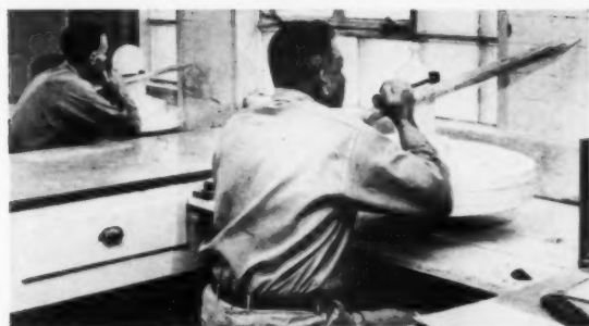
Three phases in the making of Coors chemical porcelain: (left) clay models mounted on turntables are shaped by hand to precision tolerances; (below) perforated "dissolving" cones are hand-dipped in porcelain enamel; (below left) laboratory ware is fired by being passed slowly through a circular tunnel kiln, where temperatures up to 3000° Fahrenheit are maintained.
