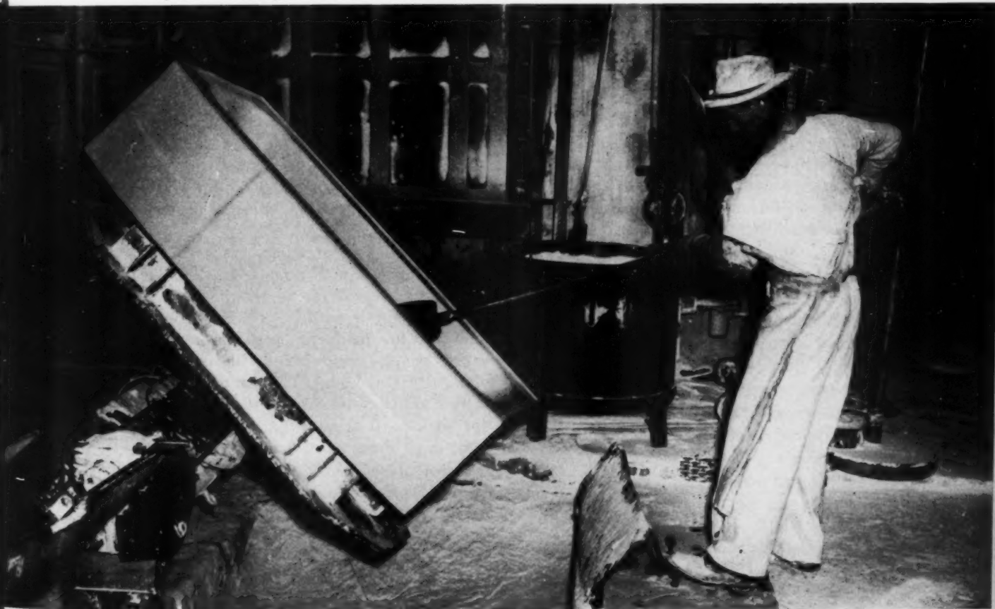
Porcelain enamel powder is "dredged" on a red hot metal bathtub. The coating is built up by a succession of dredging cycles.
