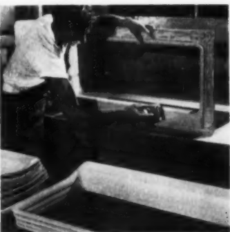
Other automotive parts made from premix are (left) automobile arm rests, placed on cooling fixture after molding to prevent warpage, and garnish molding (right) being sanded after cooling at Fabricon Products.
