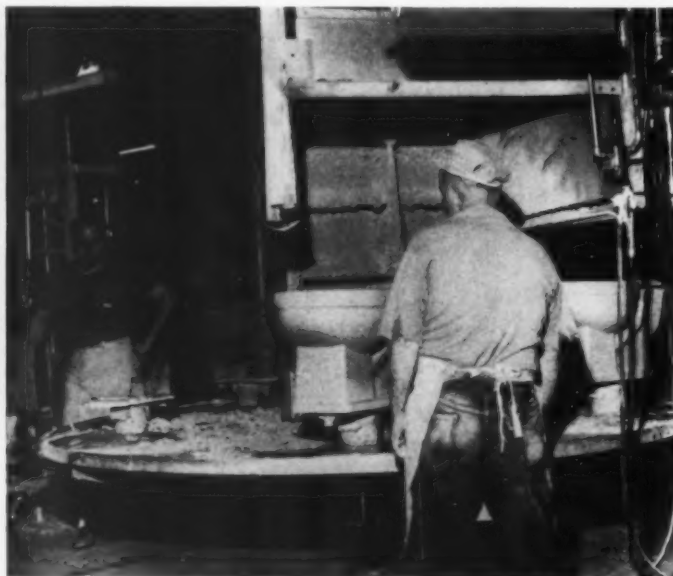
A "lazy susan" is used at Crane to speed up glaze spraying.
