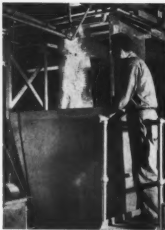
Making porcelain enamel "frit" at Ferro Enamel Corp. Molten glass (left) passes from a continuous smelter to water-cooled rollers. The sheet of compressed particles emerges from the roller (above) and falls into a vibrating hopper prior to milling.
