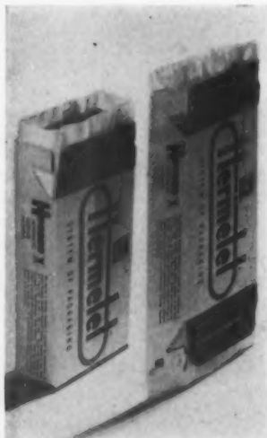
2. Hermetet is a system, originally European, of forming a carton with an integral inner liner.
