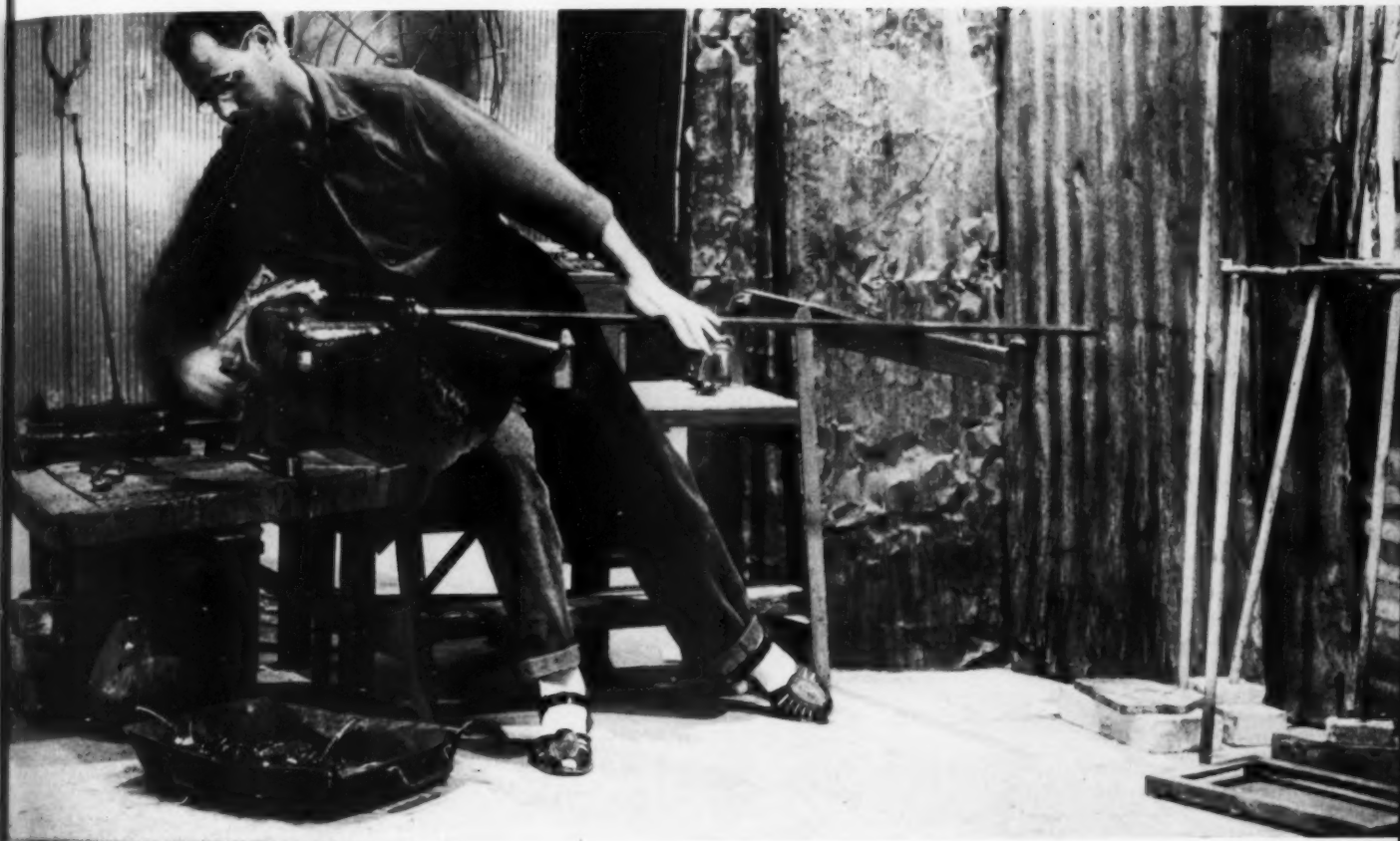
A Blenko craftsman, after blowing a hot globule of glass into a bubble, spins and shapes it according to the prescribed design.
