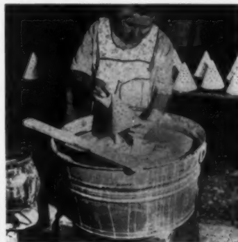
Three phases in the making of Coors chemical porcelain: (left) clay models mounted on turntables are shaped by hand to precision tolerances; (below) perforated "dissolving" cones are hand-dipped in porcelain enamel; (below left) laboratory ware is fired by being passed slowly through a circular tunnel kiln, where temperatures up to 3000° Fahrenheit are maintained.
