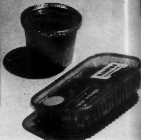
4. Left to right: low-cost styrene food containers, transparent and metallized; corrugated aluminum foil cheese container; cellulose acetate or rigid vinyl container for preserved foods.
