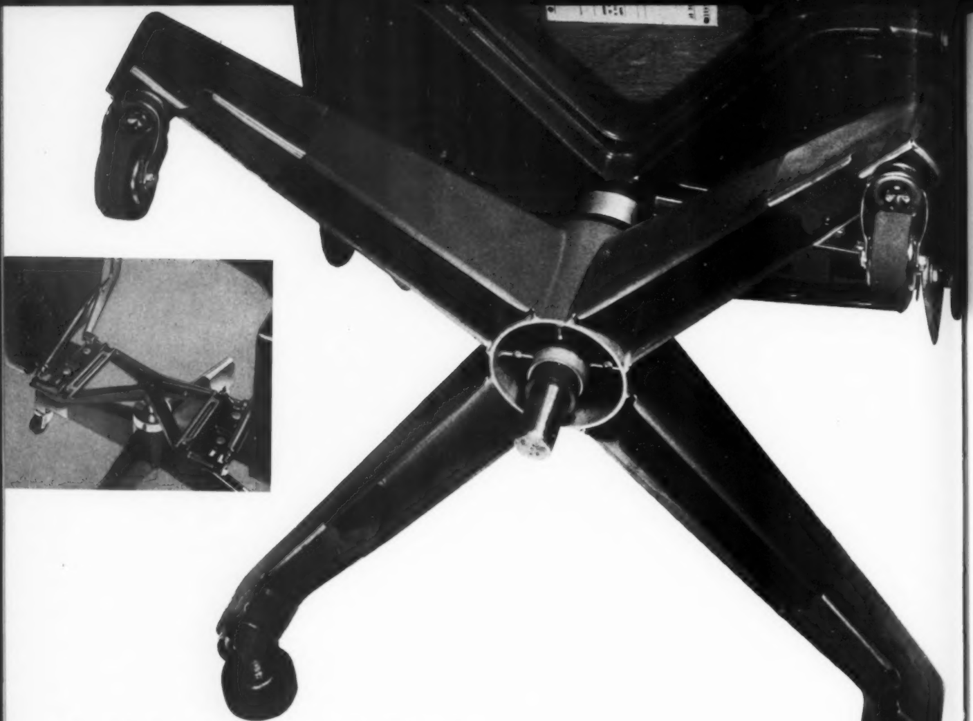
Maze of tracks on die-cast aluminum spider (Sterling Brass Foundry, Elkhart, Ind.) indicates the complexity of mechanism needed for complete adjustability. Underside of zinc die-cast one-piece base shows how edges have been rolled for a smooth, snag-proof finish. (New Products Corp., Benton Harbor, Mich.) Back supports are chrome-plated stamped steel. (Dayton Rogers Co., Minneapolis.)
