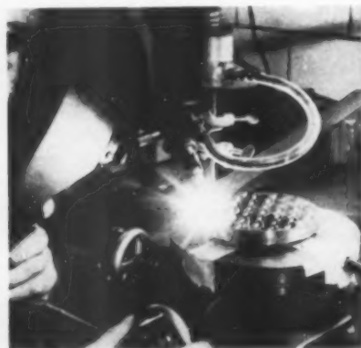
New precision is given to metal shaping, machine tooling and welding in these remarkable machines. Above is the Lockheed process of shaping sheet metal to high tolerances by means of a "two-way-squeeze" in forming. Below left is the Griscom-Russell torch for delicate welding of tubes with thin walls, and at right the electronic controls of the Inchworm Motor that guides machine tools.
