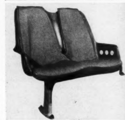
Budd engineers redesigned four-wheel truck, saving 25,000 lbs. per car (top). Reinforced plastic parts include steps, car skirts, battery boxes, one-piece lavatory unit and seating, upholstered in vinyl foam.
