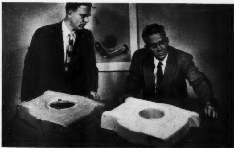
Laird Covey and W. E. Sullivan compare clay and plaster models. The new design relieves any tendency to wrinkle at the slope of the rear deck by the use of a ribbed area which also accents the spiral section.
