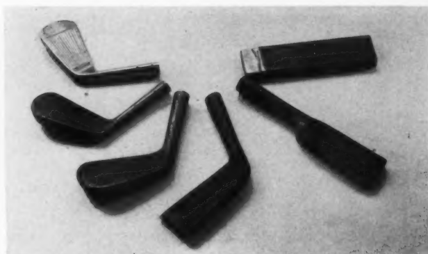
A slab of iron is worked and formed to become the head of a golf iron.
