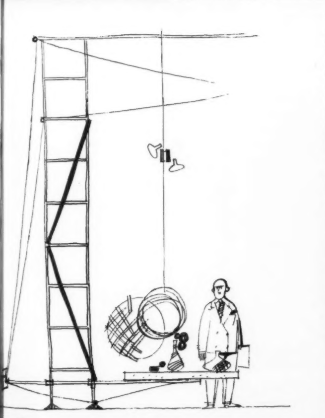
Section shows how vinyl strips were stretched from projectors, which was also designed to support cantilevered tables.
