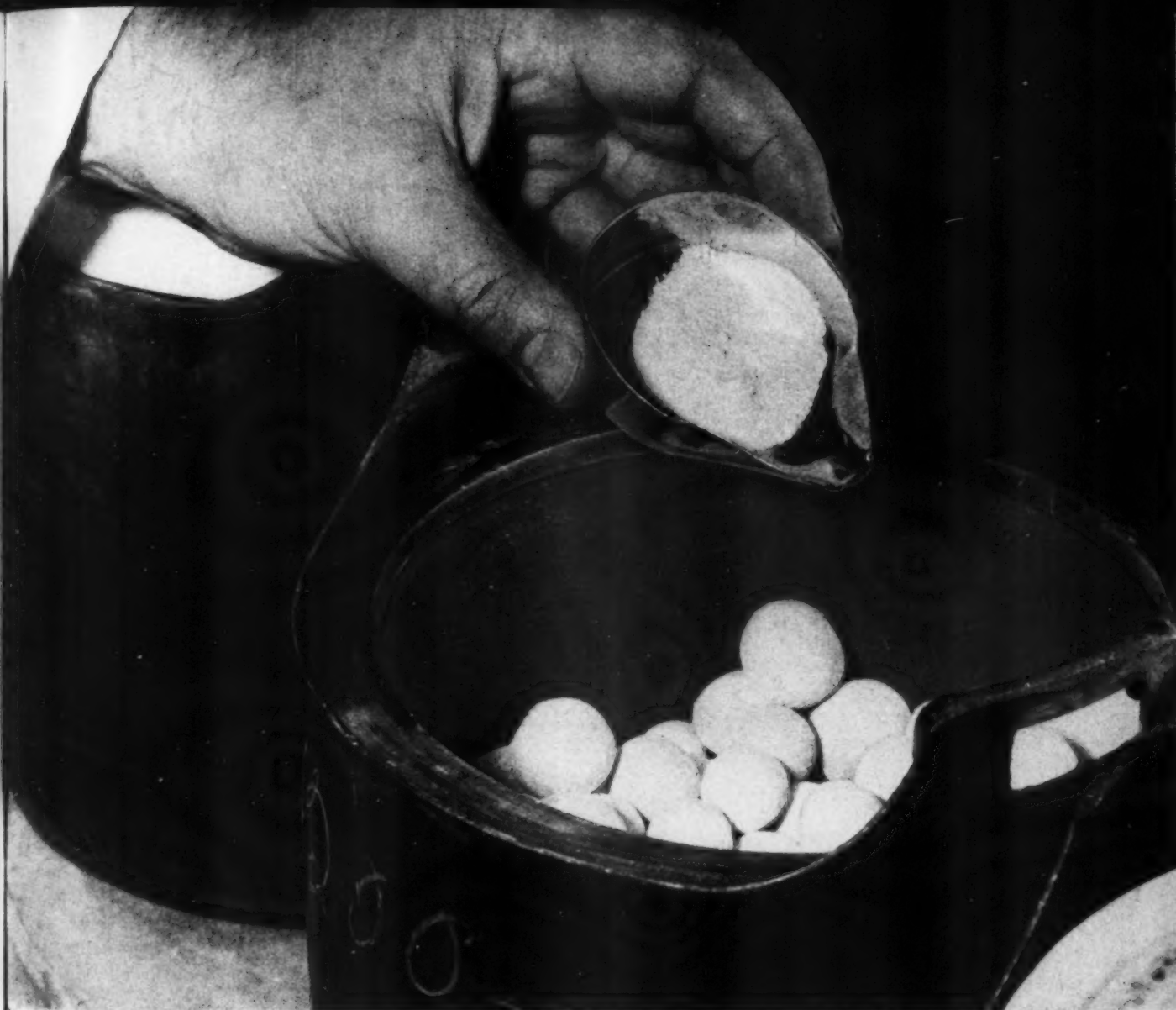
Small amounts of molding compound and pigment are mixed in a laboratory ball mill—a step in the formulation of a new color.
