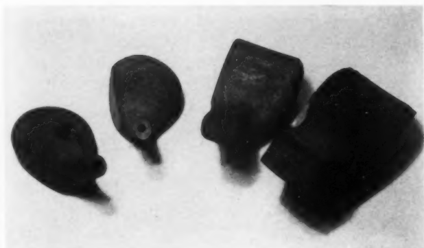
The wooden head of a driver takes shape in four steps from a clumsy block to an efficient implement.
