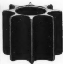
This end plug for aluminum tubing used in furniture was produced completely by upsetting or cold-heading a small diameter aluminum bar. The original plan called for it to be machined from a much larger bar. By cold-heading much material and machine time were saved.
