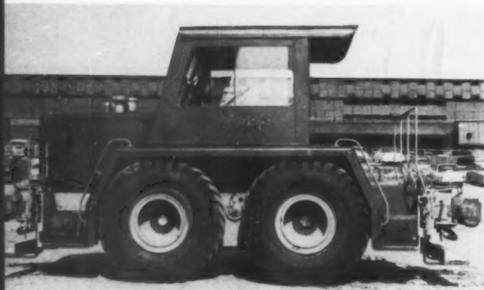
185 Switchmobile LeTourneau-Westinghouse Co., Peoria, Ill. Painter, Teague & Petertil, consultant designers Light machine to switch railroad cars in city areas replaces heavy switching locomotive. Rubber tires are quiet, save wear on streets.
