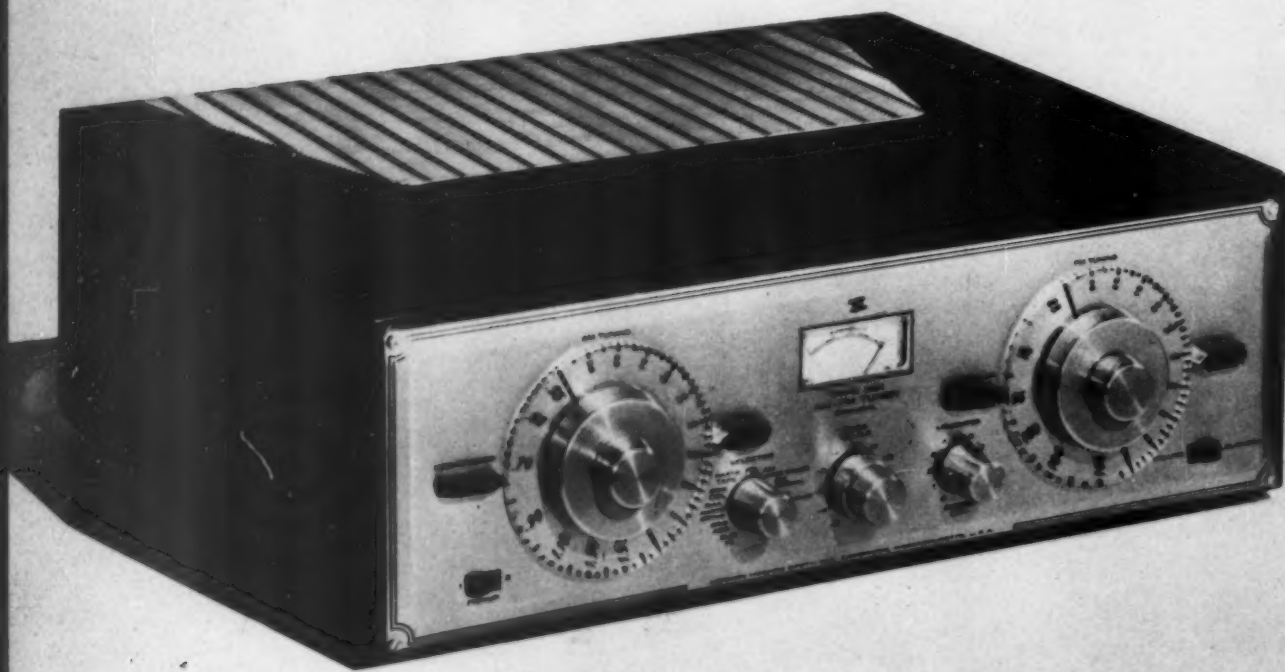
11 331-B AM-FM stereophonic tuner H. H. Scott, Inc., Cambridge, Mass. V. H. Pomper, staff designer Two separate tuners (AM and FM) in one chassis using planetary drive tuning for accurate binaural radio reception. Each has concentric knobs for quick sweep of band with outer knob, fine tuning with inner one.
