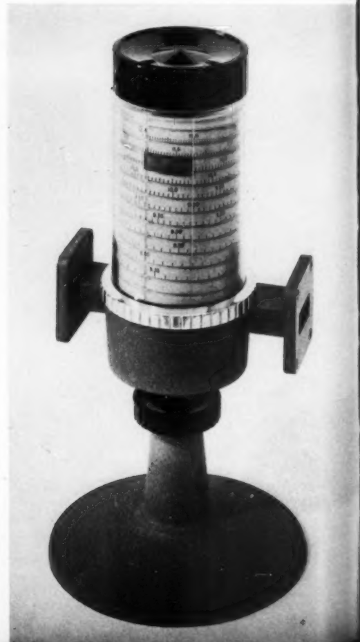
200 Frequency meter Hewlett-Packard, Palo Alto, Calif. Carl J. Clement, Jr., staff designer Accurate measurer of microwave frequency; positioning knob turns calibrated cylinder for direct readings.
