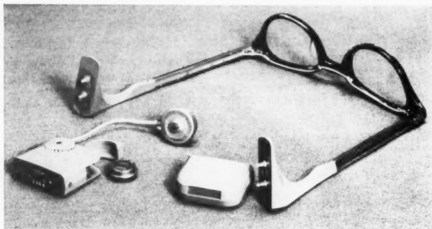
218 Hearing aid Radioear Corp., Pittsburgh Peter Muller-Munk Assoc., designers Weighing 1-ounce complete, hearing aid with aspirin-size battery, high- sensitivity mike and transistorized amplifier, fits on eyeglasses.
