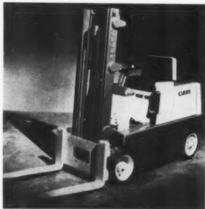
182 Fork-lift truck Clark Equipment Co., Battle Creek, Mich. Harley Earl, Inc., consultant designers Materials-handler has auto-like controls, complete access to engine by raising hood under seat.
