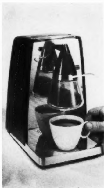
55 Automatic instant coffeemaker Charles Newman Company, Northfield, Ill. Latham-Tyler-Jensen, consultant designers Rotation of Bakelite dispensing head deposits powdered coffee, tea, etc., in cup, activates element that heats cold water to boiling and meters it into cup. For restaurant, office, home use, makes up to 120 cups/hour.
