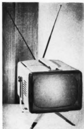
15 “Personal” television receiver RCA-TV Division, Camden, N. J. Henry Rundle, Manager, Product Dev. Smallest-screen set on the market (8½”) weighs 22 lbs., collapsible antenna; swivel base on 4 legs to adjust viewing angle.
