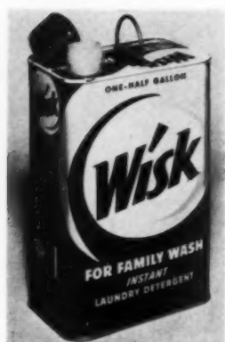
236 Detergent cans Lever Bros., New York Lippincott & Margulies, designers Pt., qt., 1/2 gal. steel (U. S. Steel, Bethlehem) cans (American Can, Continental Can); fitted with polyethylene (duPont) spout and polystyrene cap with specially angled serrations.
