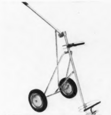
213 Golf cart Eldon Mfg. & Eng. Co., Milwaukee, Wisc. Donald V. Foerster, designer Cadmium plated frame and handles (Nikoh Tube), aluminum wheels (Gleason) shipped knocked-down; telescope assembly.
