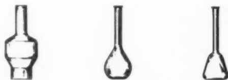
Complex shapes (above) are not desirable for machine blowing operations as the glass cannot be blown out fully with consistent thickness. Shapes below are well-proportioned and simple, making machine blowing possible.
