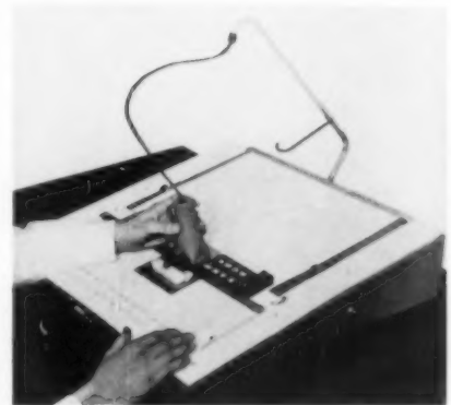
↑ Mergenthaler Linotype and The Davidson Corp. have become the exclusive distributors of ProType, a new machine that sets display type and headlines photographically. Type is produced on photosensitized film and paper by contact printing from negatives called ProFonts.
