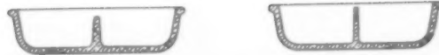
Desirable design (left) for pressed ware has sections thick enough so that glass will retain its heat and fluidity as it fills the mold. Undesirable thin sections are on the right.
