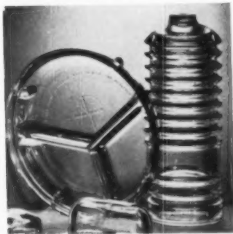
Typical machine-pressed ware reflects characteristic glass thicknesses and depth effect.
