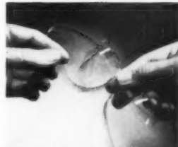
Thin, flexible ribbon glass is used in electronic components
