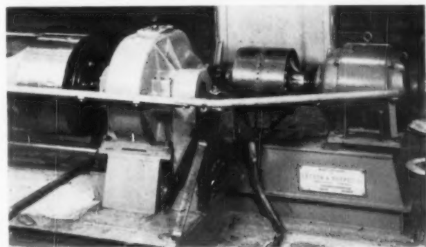
Industrial application of Tormag Magnetic Drive in Canadian plant shows unit installed between motor and load.
