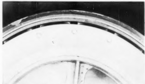
Front view of assembled magnetic drive shows tiny airgap between magnets and copper facing of bimetallic rotor.
