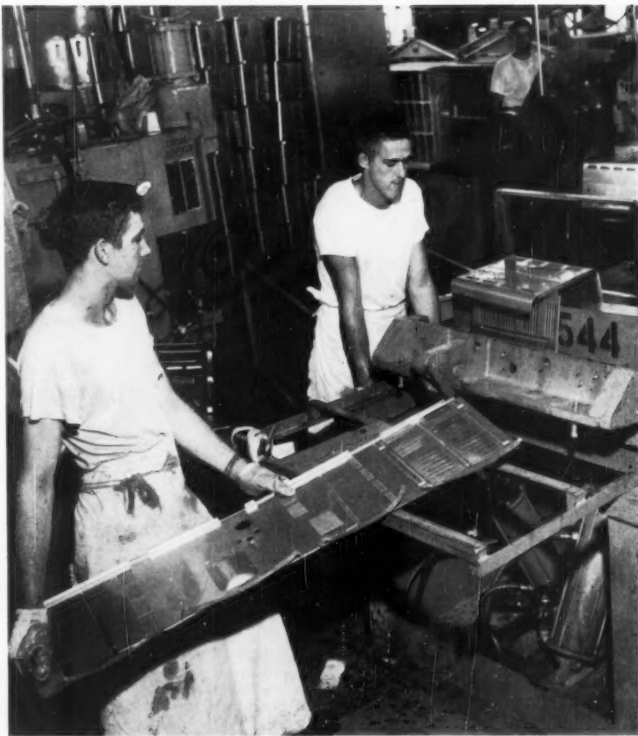
Metal cabinets (both aluminum and steel are in production) for the 10" Admiral portable are shown in the forming operation. Aluminum wraparounds are one of the important weight-saving features of both the Admiral and G.E. personal receivers.
