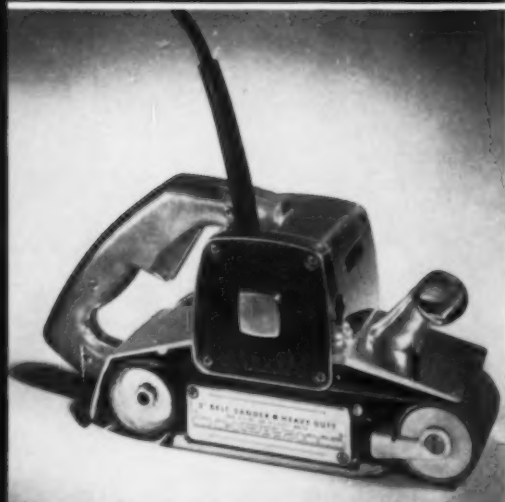
The Stanley belt sander, one of two sanders in their new line, and (above) the clay model from which it grew. The sketches (left) show how the belt sander can be used in horizontal or overhead positions.
