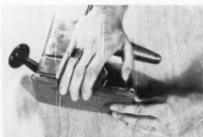
A tiny lever releases the clamp bar for sandpaper insertion at each end in the orbital sander. Clamp bar raises to lock paper in place for sanding.
