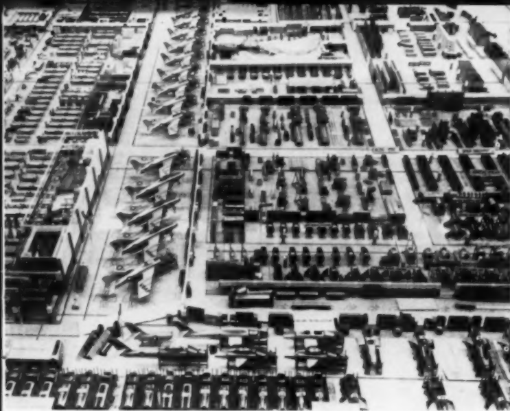
Model of plant layout for aircraft industry helps industrial engineers to organize complex plant operation. Model by Atkins & Merrill.
