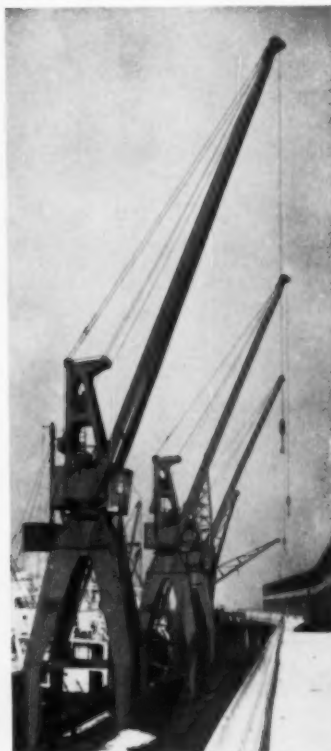
Steel-plate jib construction is used for easy maintenance, but gets more pressure from wind, is heavier than latticed jibs (left).
