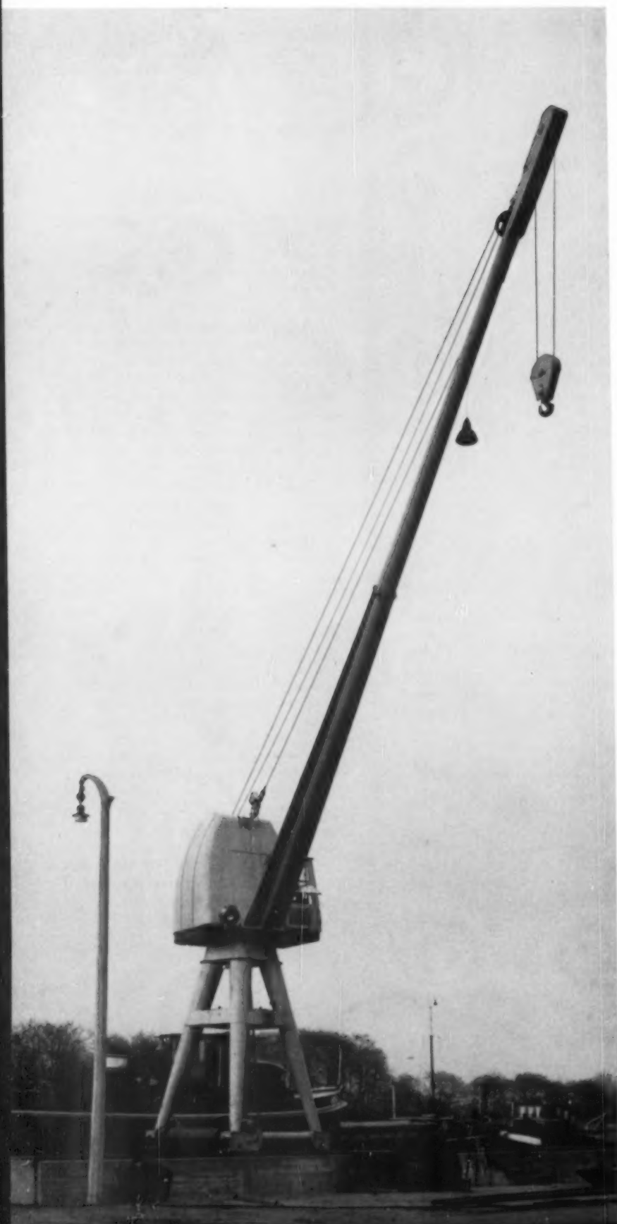
Spidery shapes of cranes using telescoping tube jibs, though they may appear more interesting than practical, are actually more powerful than others of their size. Hydraulic system allows arm to reach any point within its maximum and minimum radii. Tubular arm harmonizes well with curved welded surfaces of housing.
