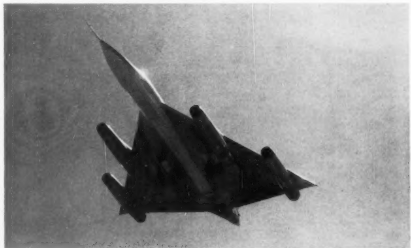
AMERICA'S FIRST supersonic bomber, the B-58 Hustler, combines delta-wing construction and four General Electric J-79 jet engines for operation at altitudes above 50,000 feet. Built by the Convair Division of General Dynamics Corporation, the plane is 95 feet long, has a wingspan of 55 feet, and carries a crew of three.
