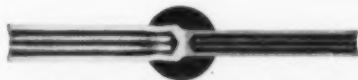
FIGURE 2. The ALCUnector consists of elongated aluminum and copper cups whose bases are butt welded together as shown in this cross section. A dielectric ball is then molded around the joint to minimize galvanic action between the two metals.
