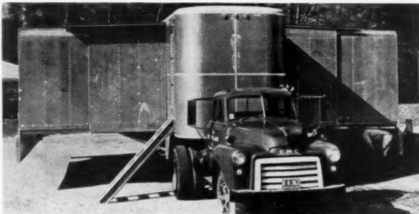
AT THE PRESS of a button, the 14-ton aluminum truck expands to five times its size. While the sides telescope outward, accordion-folded floors drop into place to form a 780 square foot area. It's all done with electrically operated hydraulic and chain drive mechanisms in five minutes. Made of Alcoa aluminum by the Gerstenslager Co. of Wooster, Ohio, it is suited to transporting military equipment, traveling exhibits, and even as a mobile home, the manufacturer suggests.
