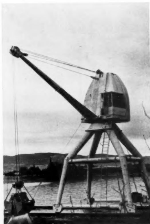
Spidery shapes of cranes using telescoping tube jibs, though they may appear more interesting than practical, are actually more powerful than others of their size. Hydraulic system allows arm to reach any point within its maximum and minimum radii. Tubular arm harmonizes well with curved welded surfaces of housing.
