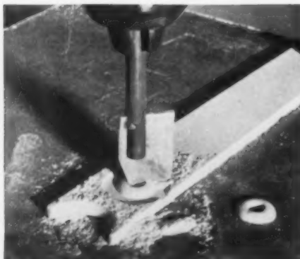
used plaster rings for grommets
