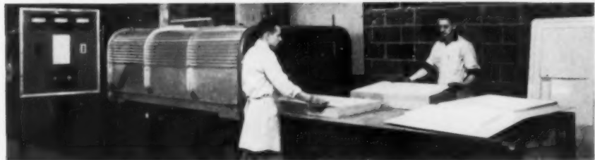
Vacuum forming plastic parts
