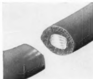
Cross section shows relative thickness of resilient coating that provides a smooth, comfortable grip for scissors handles and conforms to uneven under-surface.
