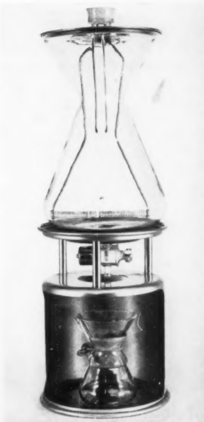
▲ Chemex Drinkwater Boiler is an entirely new solution to the problem of boiling large quantities of drinking water quickly and safely. It holds 2½ gallons of water which it can boil by electric current in about 45 minutes. Made of ¼" thick Pyrex, it has a lid with stainless steel outer rim, glass center, and molded nylon cup for attaching electric cord. Invented by Dr. Peter Schlumbohm. $125.
