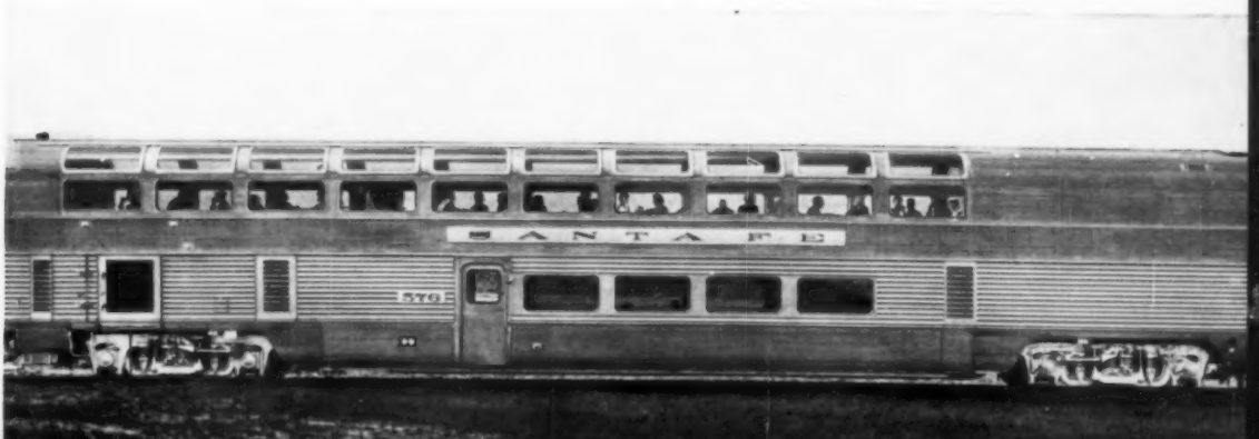
Large structures joined by Budd's "shot welding" process
