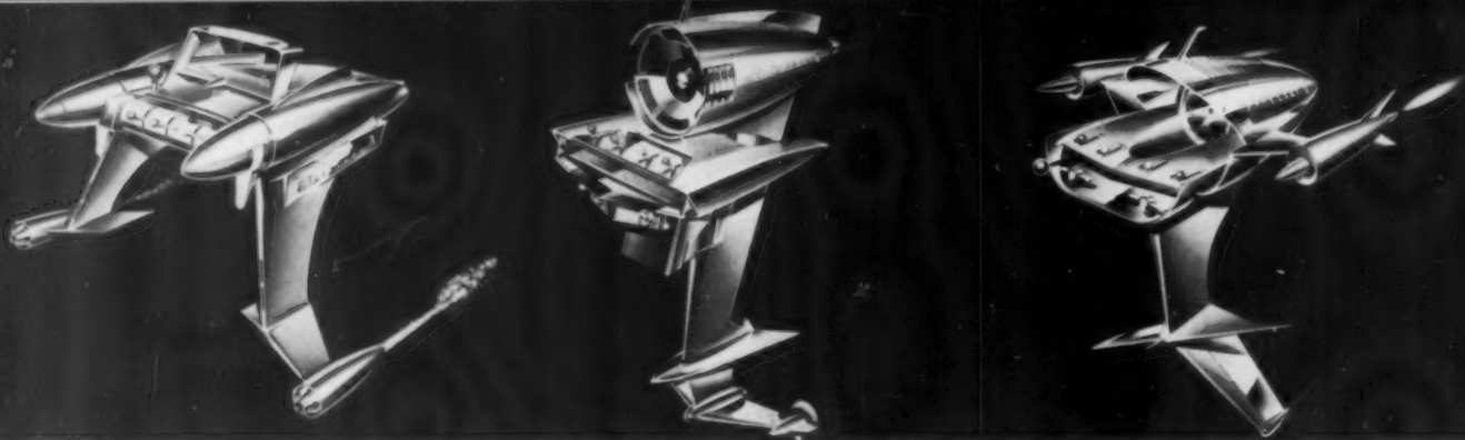
Brooks Stevens' outboard prophecies (l. to r.): Aqua Jet uses engines to pump water back at high speed through underwater jet nozzles; Turboprop gas turbine similar to jet plane motor drives twin propellers, has remote-controlled steering; Turbojet's twin exhausts thrust hull forward at high speeds with aileron-like steering controls angled for banked turns.
