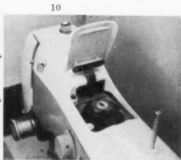
Greater control: (4) Pfaff thread tension has metal discs rather than coiled spring; (5) Morse stitch-length dial pictures stitches; (6) Necchi presser foot is calibrated on front plate.
