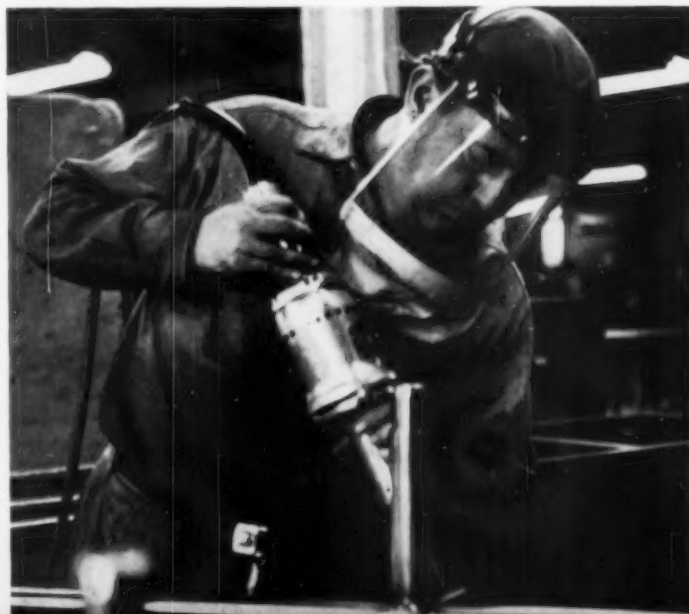
Hand grinding makes welds smooth and easy to keep clean.
