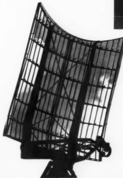
Stainless radar antenna.
