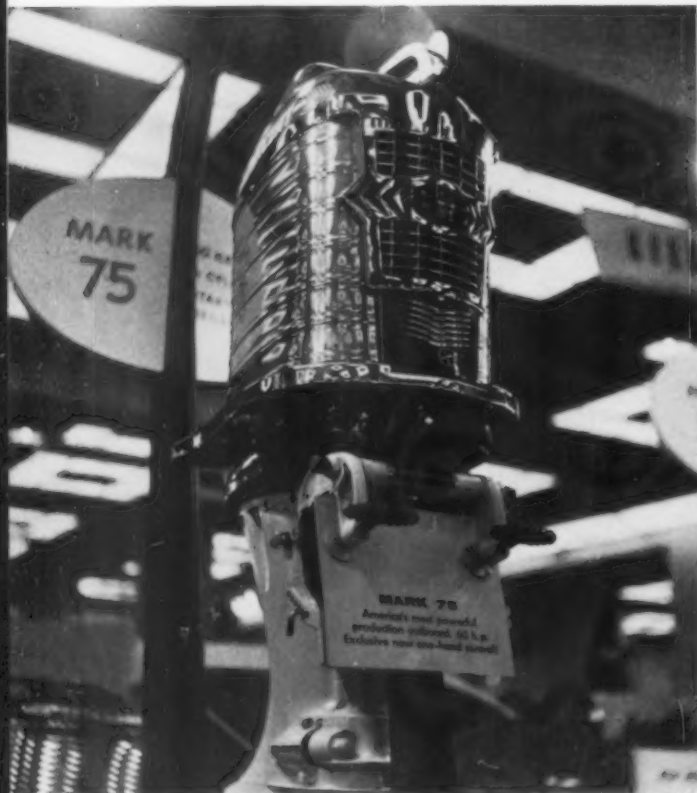
Mercury Mark 75 offers 60-hp. at relatively low weight (140 lbs.). Innovations include six cylinders (smooth-running), single lever control with direct reversing, three synchronized semi-sealed carburetors. Despite trend to yearly obsolescence, tradition of life-time durability is still strong in industry; Evinrude takes pride in its first handmade $62 model of 1909 (above); Johnson offers innovations as replacement items to protect owners.
