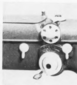
Pfaff controls (13) bypass logic for symmetry. Two polywog knobs control unlike operations; needle position lever is separated from its arbitrary 1, 2, 3 markings by large dial. In Viking (14) needle position knob points to diagram.
