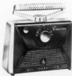
† Antenna enclosed in rotatable carrying handle brings reception from any direction to Emerson's Model 868 all-transistor portable. The ferrite-bar loop-antenna offers the equivalent of an additional stage of amplification. $38.00 price includes Miracle Wand antenna.
