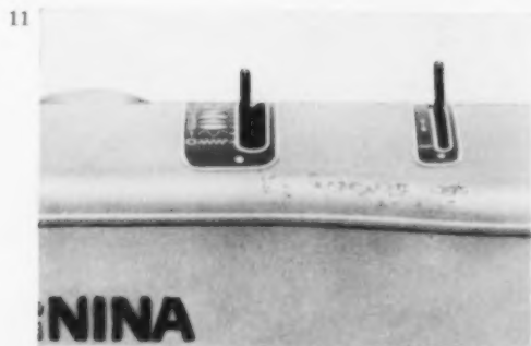
Necchi cams are assembled, put into machine (10). Built-in Pfaff cams (12) are dialed inside machine. Bernina lever (11) sets cams inside.
