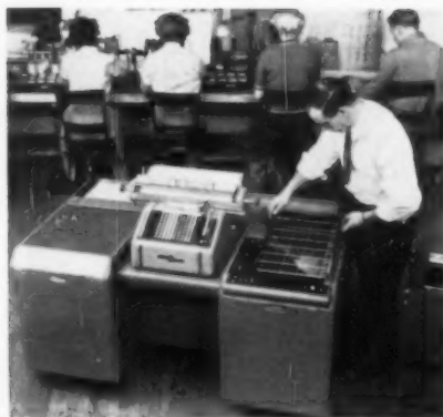
E 101 desk-size computer was Burroughs' first electronic machine, but incorporated Sensimatic input-output mechanism; developed at Research Center, Detroit Manufacturing Dept. set up special organization to engineer it for production.
