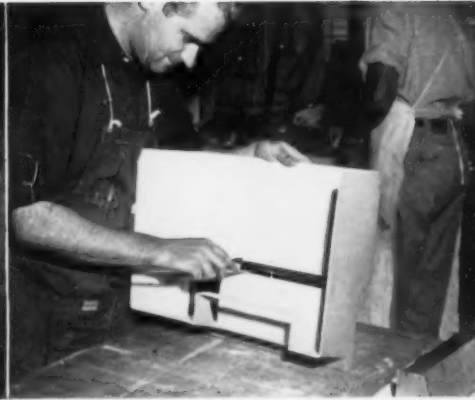
Rough Fiberglas housing, supplied by Harley Earl Inc., is refined by filing and prepared for trim parts assembly.
