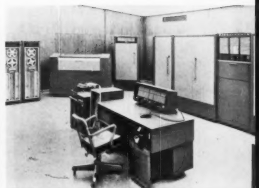
Datatron is medium-price electronic data processing system, manufactured and marketed by ElectroData Division; it includes Cardatron punched-card data hookup and Datafile auxiliary memory.
