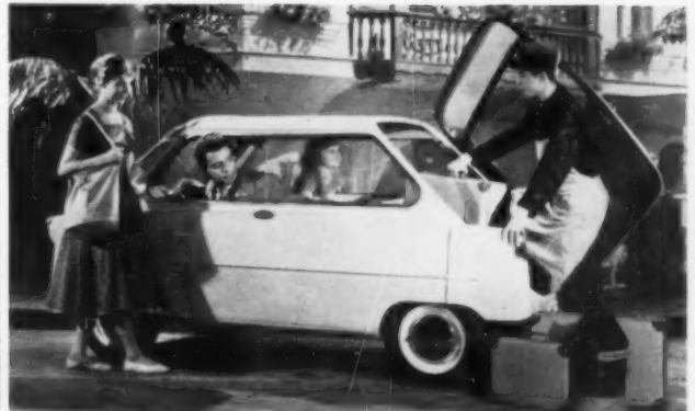
Sliding windows, identical doors, uncluttered body panels, a minimum of chrome help drop fabrication costs in the Janus. Two adults, several children, or considerable luggage can fit in the back seat.
