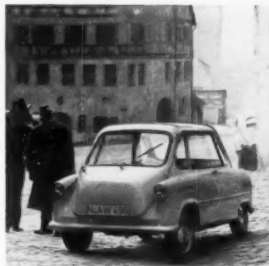
Sliding windows, identical doors, uncluttered body panels, a minimum of chrome help drop fabrication costs in the Janus. Two adults, several children, or considerable luggage can fit in the back seat.
