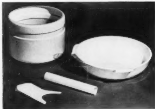
Pyroceram, Corning's new material, in its first application (top), forms the radome for a guided missile. Four types of Pyroceram—eventually there will be over a thousand—have been produced in pilot runs. Pyroceram can be made transparent, translucent, or opaque (left). The forms (below) show the material's versatility; the container was blown; the dish pressed. Regular glass-making processes are used.
