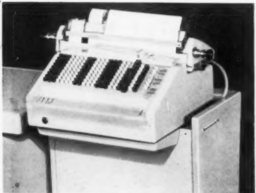
Sensitronic bank bookkeeper began the fusion of electronics with electro-mechanical techniques in product line; electronics added to Sensimatic keyboard system allows automatic pickup of old balances, automatic alignment of forms.
