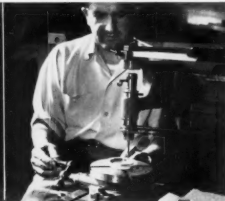
Lettering on control knob, machined out of Plexiglas block, is engraved by pantograph machine, filled with paint.
