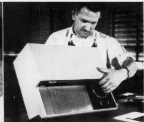
Exit chute is fastened into lower opening. Light blue-green baked enamel was color specified for production housing.
