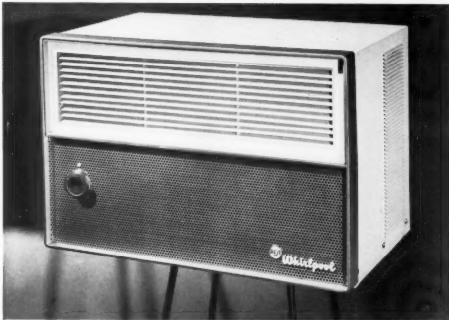
↑ Portable RCA Whirlpool Featherweight 75 weighs 90 lbs., can be plugged into any 115 volt household circuit. \frac{3}{4} hp. motor delivers 6,000 BTU per hr. Aqua enamel on aluminum, it measures 21" wide, 14" high, 14" deep.
