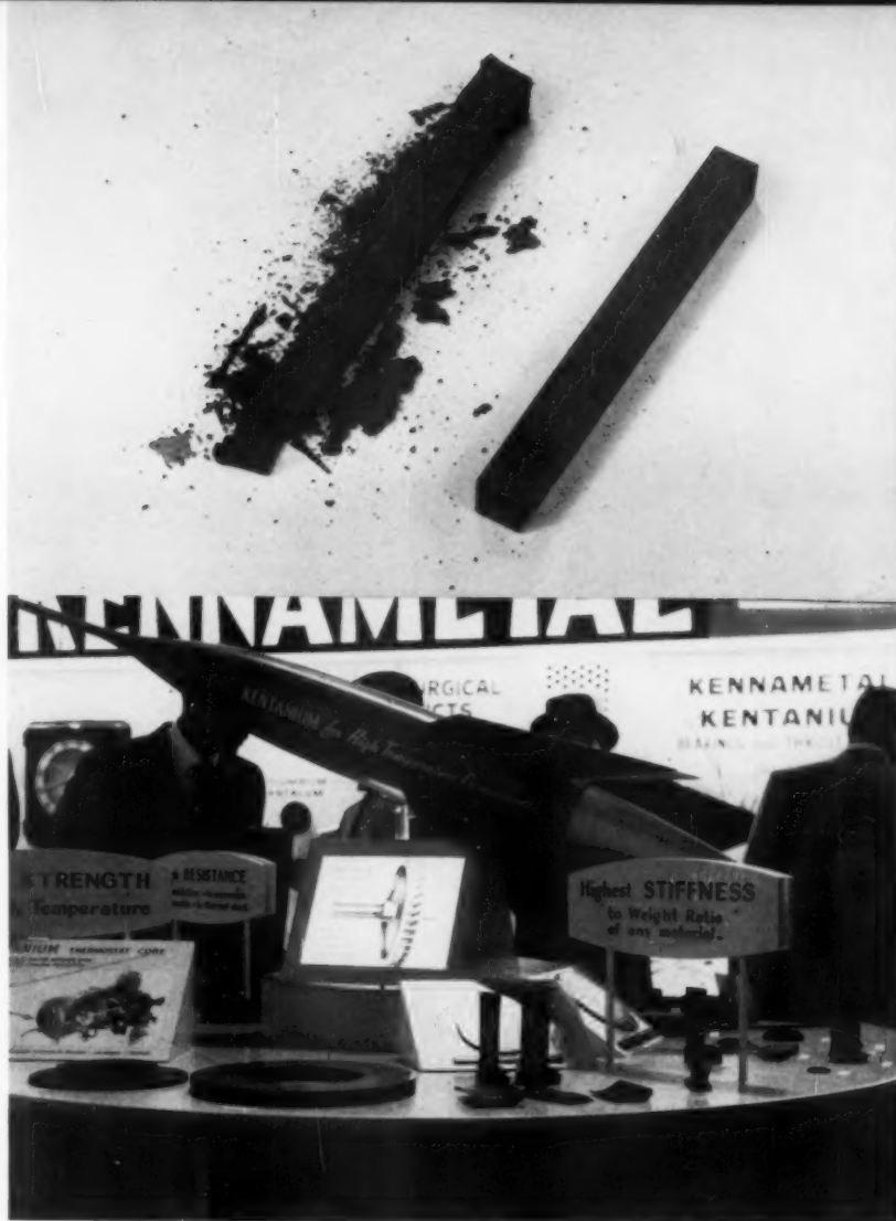
Titanium carbide, produced by Kennametal Inc., Latrobe, Pa., resists heat of 2150°F while a bar of nickel-chrome-cobalt alloy fails (top). Typical applications for Kennametal include seal rings for handling fuming nitric acid, bushings, nozzles, and valve components.
