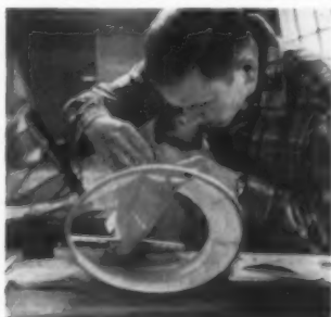
William Elzaurdia works on the fine rib keel construction of his kite.
