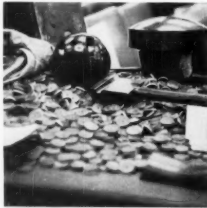
Lignum-Vitae self-lubricating wood, fabricated by Lignum-Vitae Products Corp., Jersey City.
