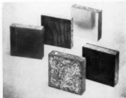
Particle board, used as corestock for veneered furniture, doors and plastic overlaid material, produced by National Starch Products, New York, is enjoying a rapidly expanding market.
