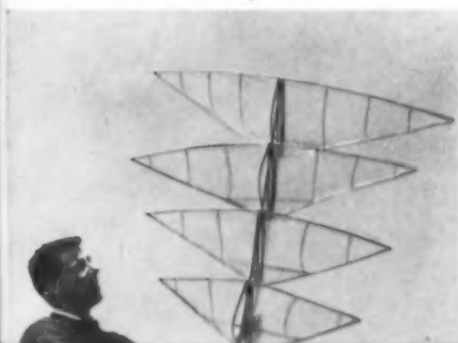
Adjustable center sections of Keats Carleton's kite could be individually set for maximum lift.
