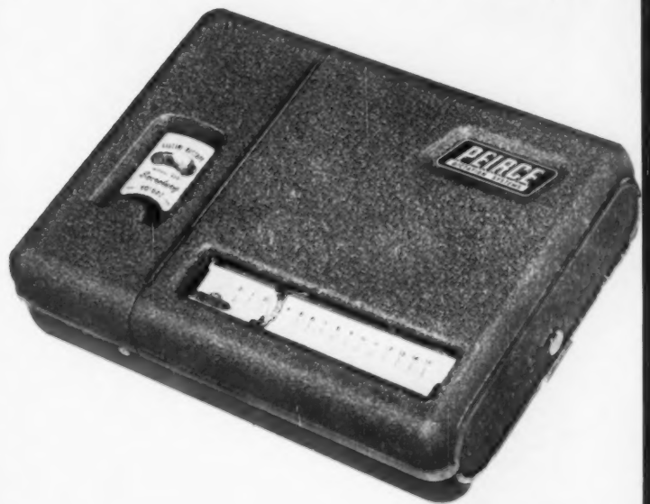
↑ A transistorized dictating machine, by Peirce Dictation Systems, the size of a book and weighing 4½ lbs., operates from self-contained batteries or line voltage. Transistorized record-and-playback amplifier has made for a hum-free size-reduced recorder-reproducer (left) designed by RCA for hi-fi music systems and industrial sound systems.
