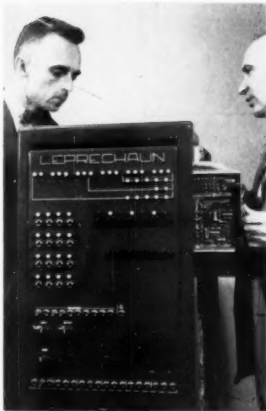
Use of 5000 transistors has made possible the small size and low power requirements of Bell's new electronic brain.
