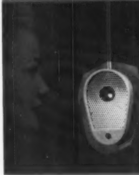
Front door camera lens permits caller to be seen on bath or kitchen
