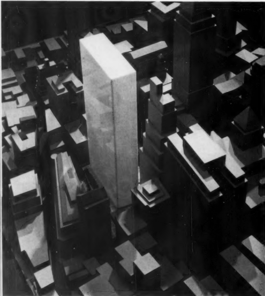
First model expression of new Chase Manhattan Bank building (white block above) and surrounding downtown Manhattan area, was followed by sectional model of base and lower floors (right) to determine fenestration and other details. Ted Conrad (in center, right above) carried through project in Jersey City shop.
