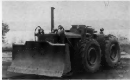
Tournatractor, before being remodeled by LeT-Wesco, had perforated grille (subject to clogging) and projecting lights.
