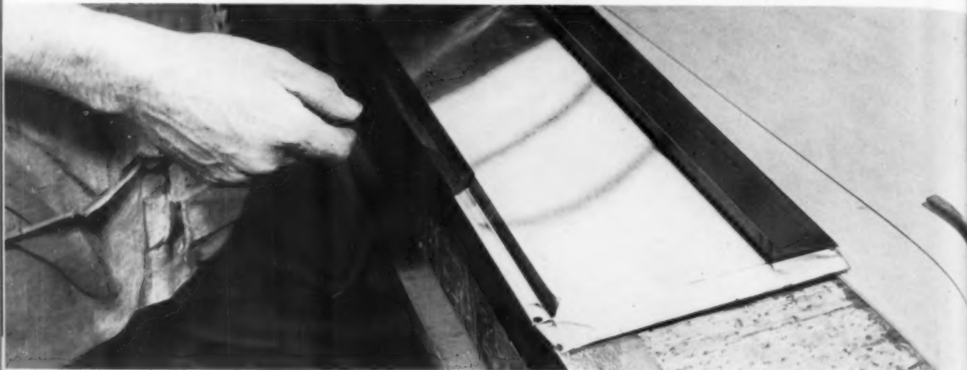
Strippable coating (Minnesota Mining and Mfg. Co.) protects stainless steel during fabrication.
