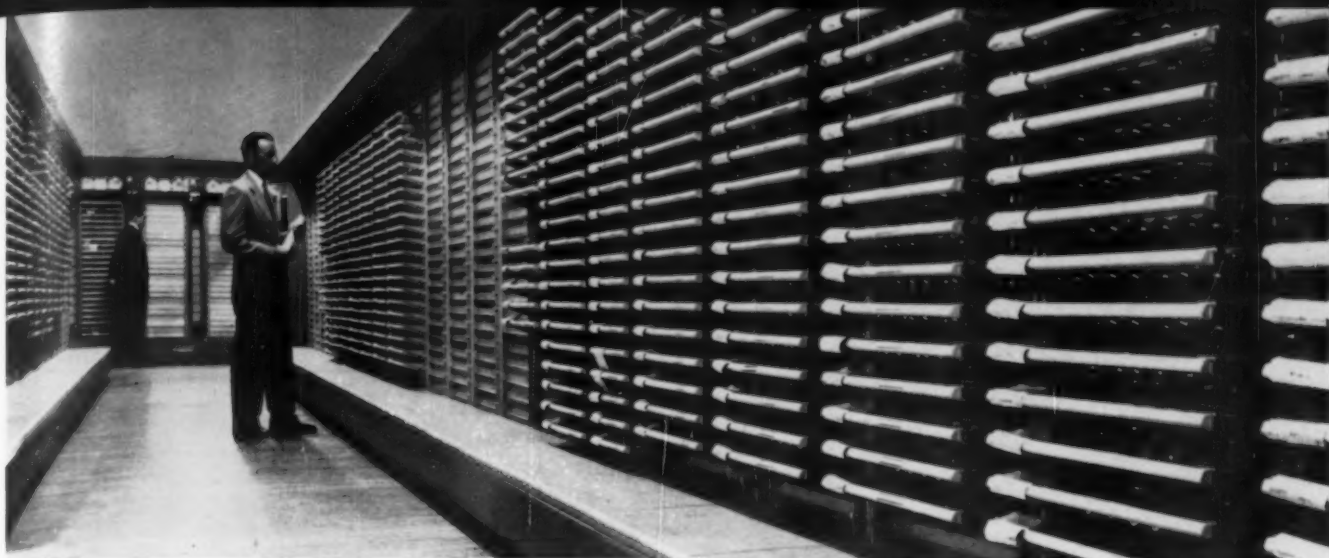
At heart of SAGE computer are rows and rows of frames made up of identical sections in which basic units—pluggable units—are stacked like shelves. Each unit performs a logical function.
