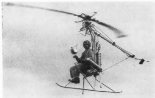
Roto-Craft "Pinwheel" is powered by rocket engines.
