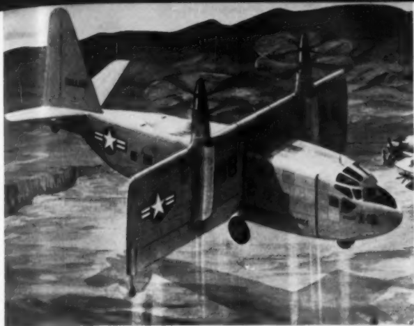
Tilt-wing airplane by Hiller changes attitude of wings for take-off, landing, and forward flight.
