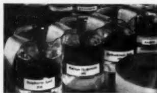
CHEMICAL RESISTANCE. "Mylar" film is unaffected by oils, grease . . . most acids and alkalis, moisture and solvents.
