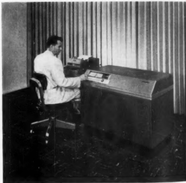
Complete LGP-30, being fed from Flexowriter, is desk size.
