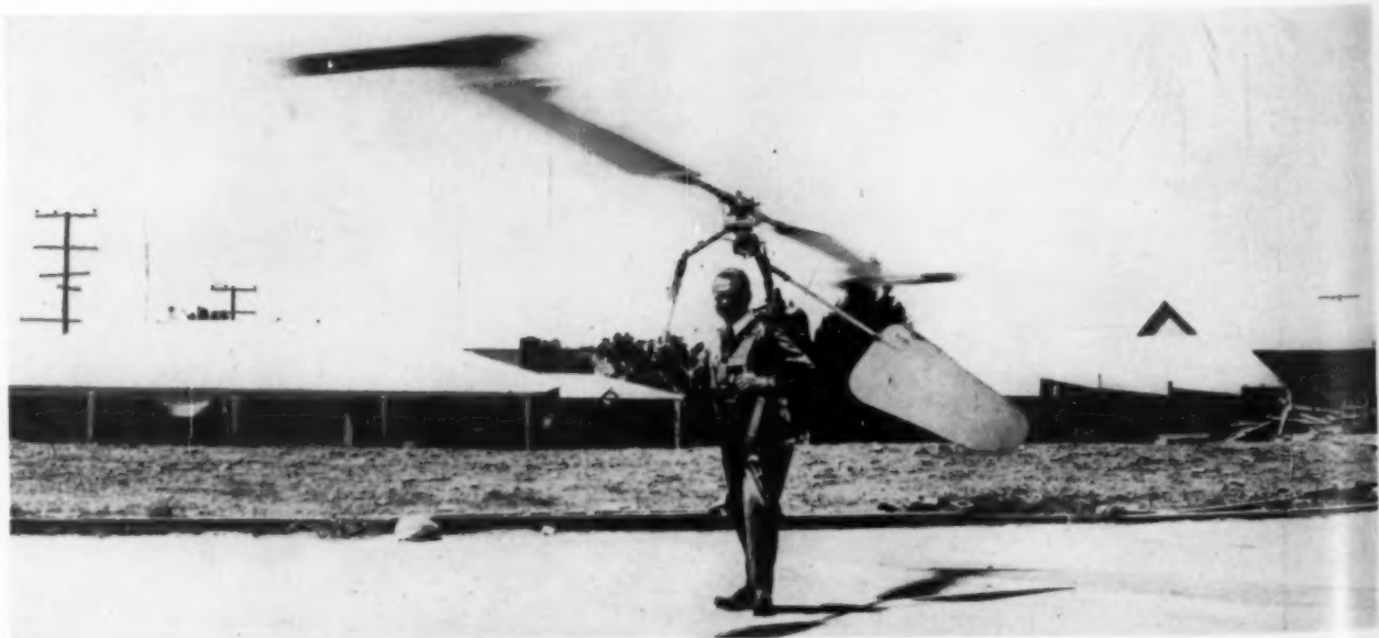
The pilot's feet are the landing gear on the Gluhareff machine.
