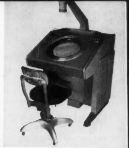
Design of a third SAGE console—the mapper console where incoming radar signals are first received—was straightforward, involved no wooden model. Sheet steel prototype served as design as well as production engineering model.
