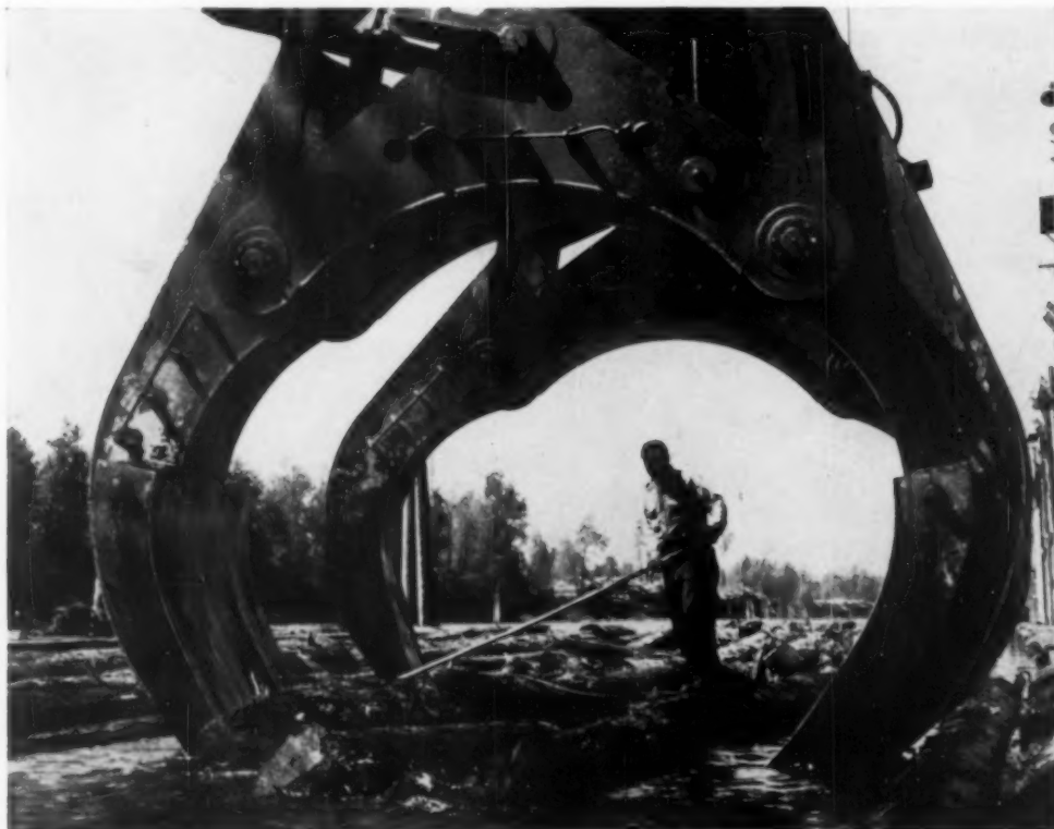
Fifty-ton Berger crane was originated by Crown-Zellerbach engineers at its Camas, Washington mill.
