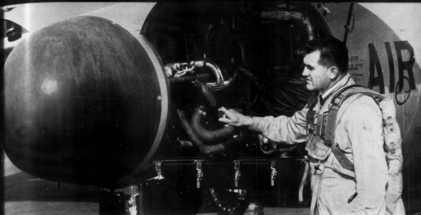
Hughes fire control system installed in nose of F-102A. Dome in front contains radar antenna.
