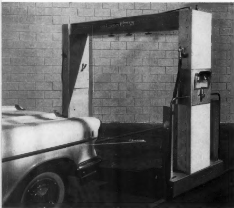
Mobile car wash machine can be operated by one man in three automatic operations, does complete job in ten minutes; Merendino-Greene, for California Car Wash Systems, Inc.
