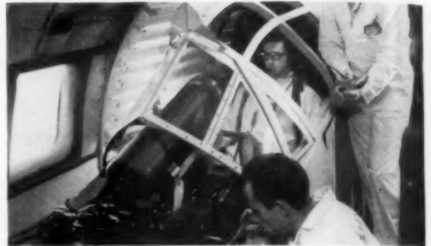
Flying laboratory: F-102A cockpit inside larger plane for in-flight testing of Hughes-Convair fire control system.
