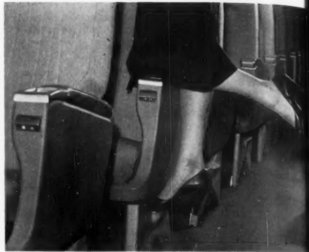
Step for stewardess makes it easy to reach hatracks without leaning over passengers.
