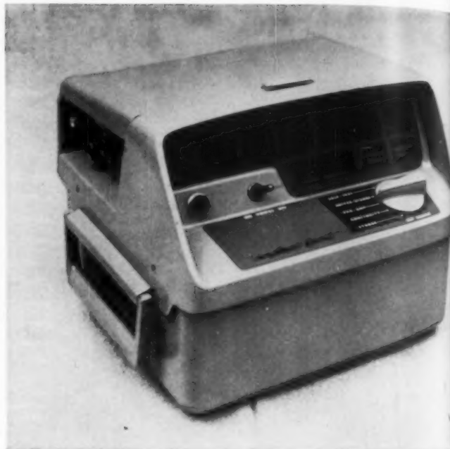
Portable analyzer for Aerojet test equipment for Lockheed F-104 interceptor fire control system uses visual presentation, simple controls.
