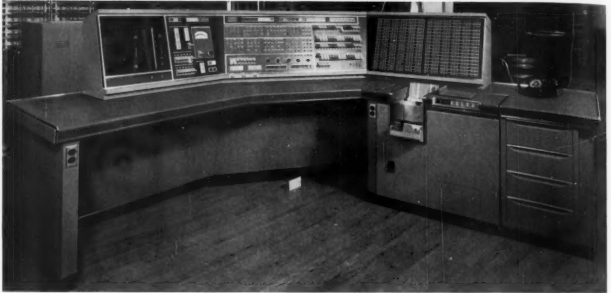
Original design concept for operation console was based on one-man operation. Wooden mock-up (left) followed cardboard mock-up study for panel locations. Sheet metal full-scale model (below) incorporated changes suggested by design committee.
