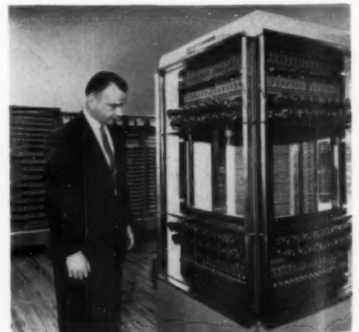
Fundamental section of electronic brain is the magnetic core memory where all SAGE data is stored. Unit was left uncovered for easy replacement of tubes and other parts.
