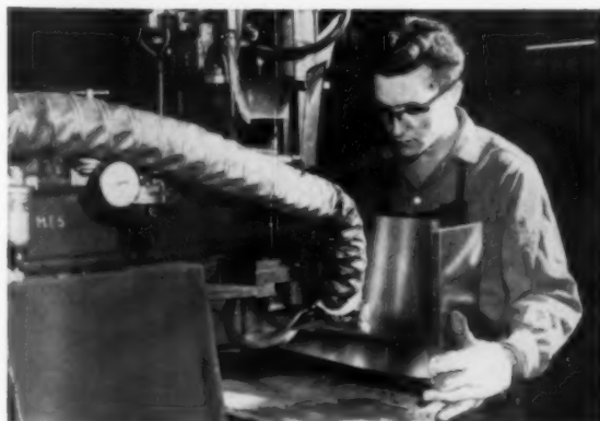
Breadbox body frame is spot welded to the preformed bottom and back pieces, with no visible oxidation. Parts then move to assembly.
