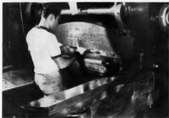
Edges of Nickeloid chrome-steel sheet are turned up \frac{3}{2} " in forming press. Nickeloid is easily worked with standard methods.
