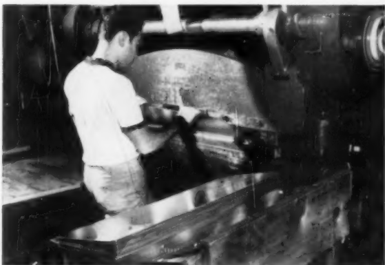
Edges of Nickeloid chrome-steel sheet are turned up \frac{1}{2} " in forming press. Nickeloid is easily worked with standard methods.
