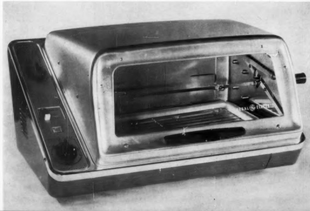
98 Portable rotisserie-oven General Electric Company Housewares & Radio Div., Bridgeport Carl N. Johnson, R. H. Koepf; Donald L. McFarland, Manager of Industrial Design Aluminum (Reynolds) tilt-top lid, Bonderized baked enamel on steel lower shell, nickel-chrome-plated steel inner liner.
