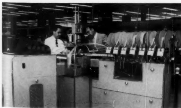
D IBM's automatic Programmed Component Assembly System.
