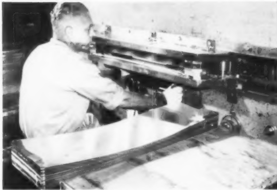
Sheet of Nickeloid chrome-steel that will be used for breadbox is blanked, with punch-out perforations for ventilation and indented shelf supports. Uniform pre-plated finish reduces rejects.
