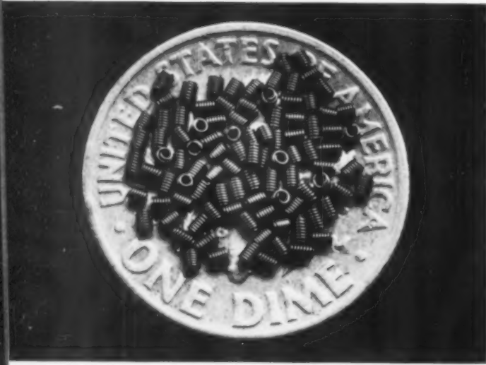
A straightforward demonstration of the size of these miniature springs is made by grouping them on the very familiar dime.
