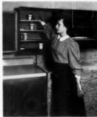
First stage of General Electric's design testing was measurement of maximum reach-in for average housewife's height. Test model of wall refrigerator was crude cardboard shell with adjustable shelves; more refined models in wood and plaster were used at later stages.
