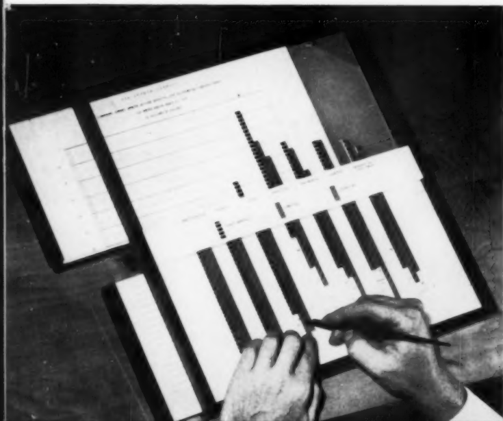
Planoscope's Bar-Graphmaster has movable plastic bars in a variety of colors and patterns that can be readily moved into position (below) and locked for presentation or reproduction (above).
