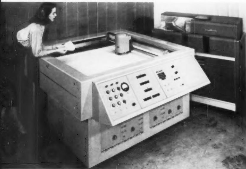
The Benson-Lehner Electroplotter works in conjunction with an IBM card punch machine to plot curves automatically. American Chart Service self-adhesive tapes are fed from a cartridge onto almost any surface.
