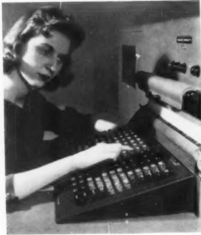
Trained typist transcribes engineering data from planning sheet to punched tape. Auxiliary master control switch for automated line of machine tools is checked.
