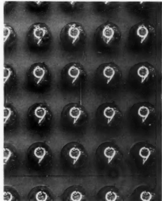
Large numerals reduce read-out errors on equipment by Computer-Measurements Corp.; below, digital read-out tubes.
