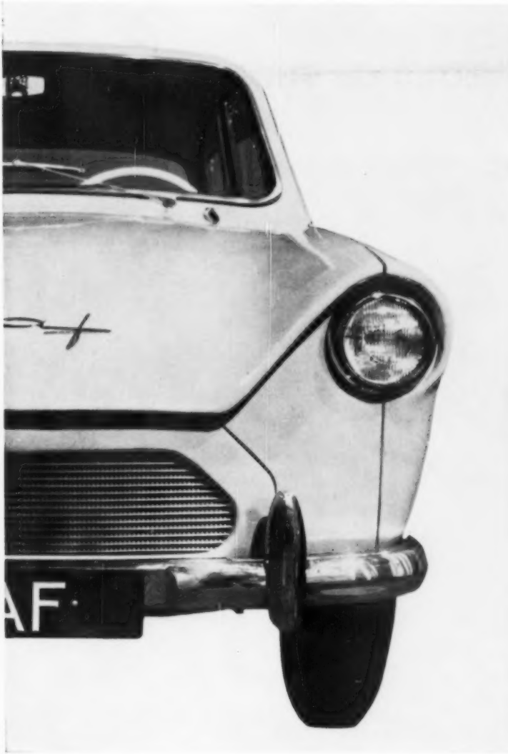
Lines are simple, chrome at a minimum in the two-door, four-passenger (142 by 56 inches) DAF. A scooped hood—possible because the engine is horizontal — helps cut wind resistance.
