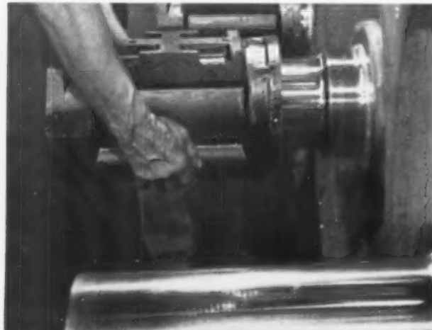
New bearing design fitted to journal. It gives better distribution of load and perfect fit. Other metals were tried, but bronze offered the best combination of characteristics for the application.
