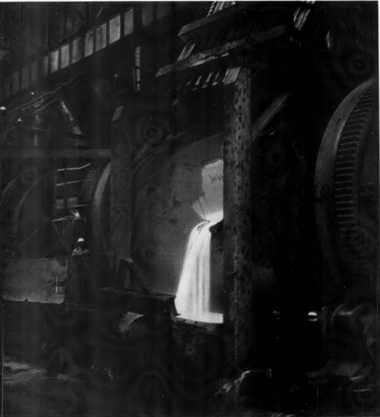
Copper poured from a converter during refining. The ankh (top right) is the ancient alchemists symbol of copper and its alloys.
