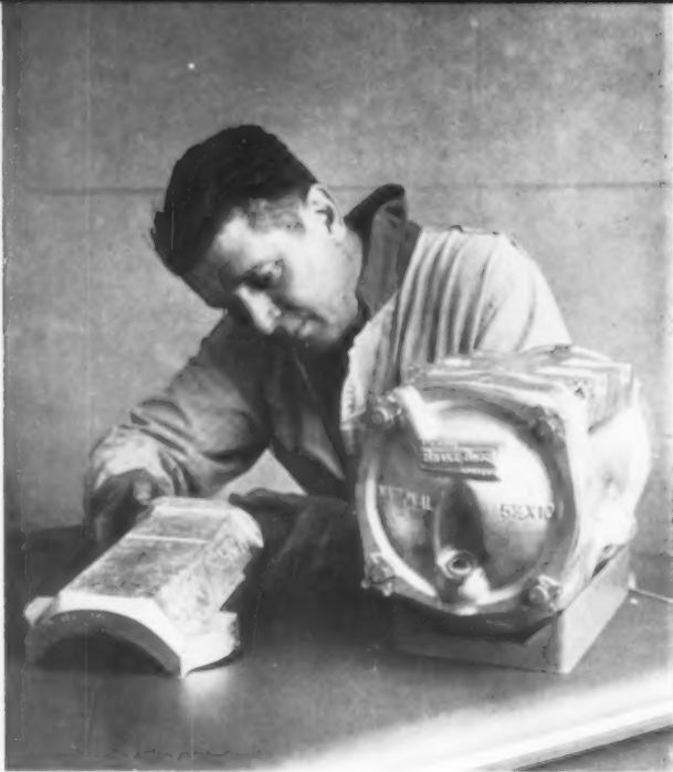
An 120° saddleback bearing is compared to 360° unit recently introduced by American Brake Shoe Co. New journal box unit for freight cars contains over 70 pounds of copper alloy, compared to the old casting that contained about seven pounds.
