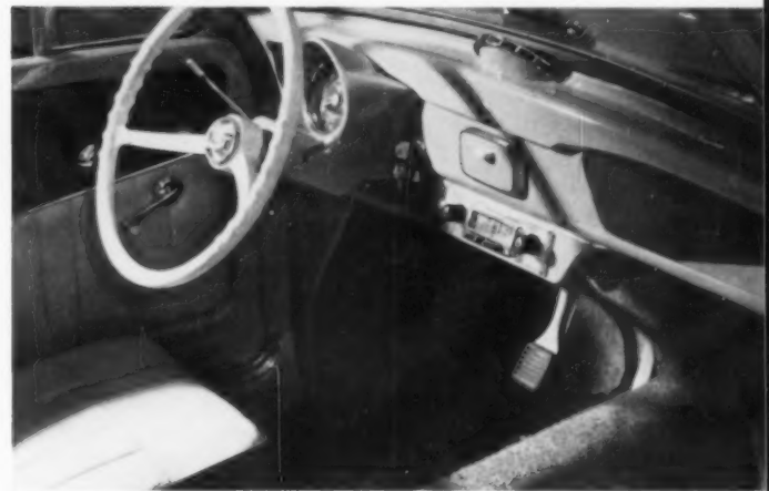
Compact dashboard carries fuel, oil pressure indicators (uncommon in this type of car). Levers below wheel control signals, horn, and headlights. Brake and gear shift are between front seats.
