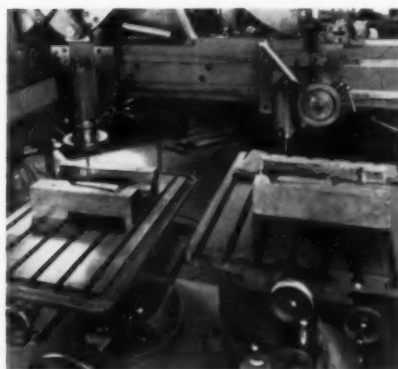
↑ Half of the cavity of the mold nears completion of rough cutting. Highly skilled technicians—and precision instruments—are needed for these operations.
