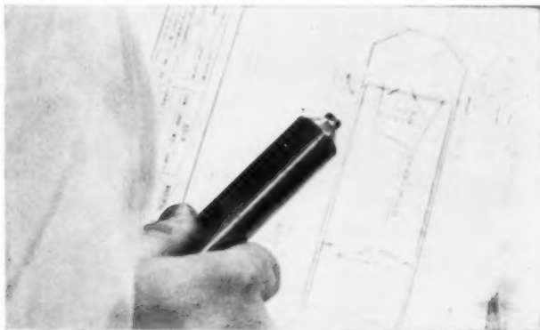
Designer checks specifications of impact extruded assembly. Blueprints can specify a variety of internal design components which can be impacted as an integrated part of the finished part.
