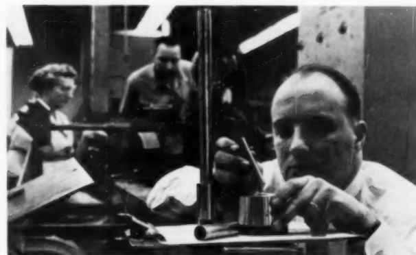
Impact extruded shape is checked against the die. The variety of flanged or cupped-end tubular shapes available for this process is unlimited. Rectangular or oval shapes may also be impacted.
