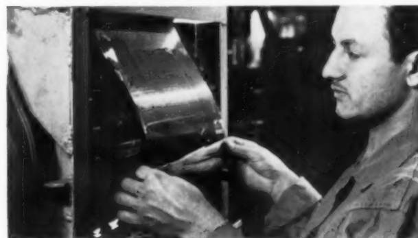
After etching, the foil is cleaned and acids are washed off in a machine specially designed by Park for this operation.
