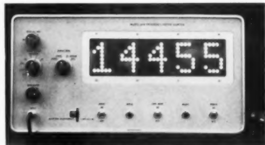
Large numerals reduce read-out errors on equipment by Computer-Measurements Corp.; below, digital read-out tubes.
