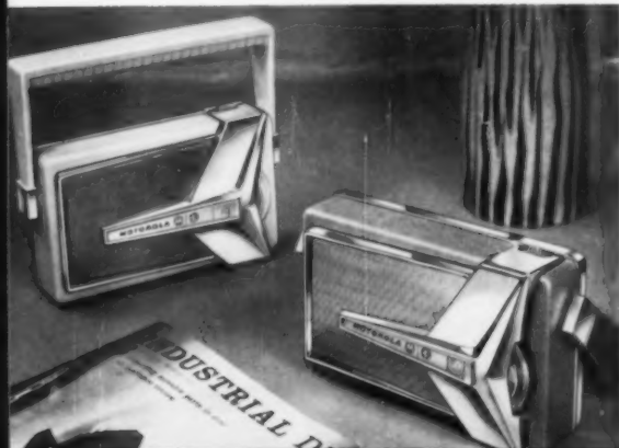
Two views of the Motorola transistor radio case in Colovin vinyl laminate. Notice in the upper view the clean edges of the punched perforations and the smooth "tailoring" of the rounded corners with no distortion of the vinyl. Lower view shows snap fastener and chassis locator flange spot welded to the laminate, die cut for handle, and hinging.
