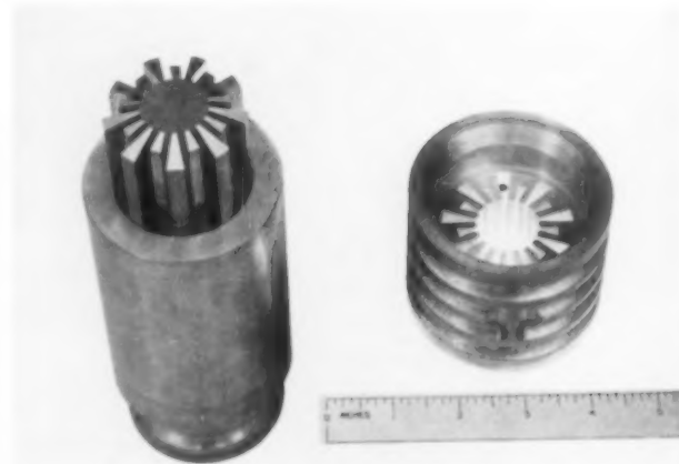
Cavity (right) assumes exact detail of hob. No further finishing operation is needed.
