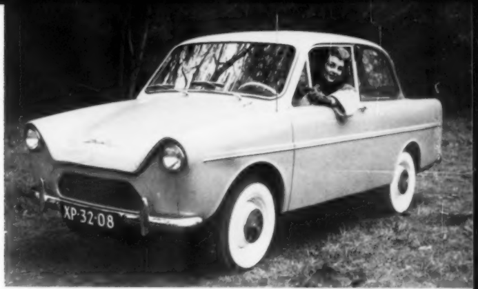
Lines are simple, chrome at a minimum in the two-door, four-passenger (142 by 56 inches) DAF. A scooped hood—possible because the engine is horizontal — helps cut wind resistance.
