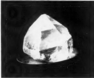
The quartz crystal seen at the Bulova booth represents the main material in quartz crystal radio filters (1D Oct. '57).
