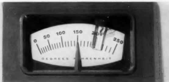
fication. Two hairlines are molded-in on the front and back for parallax sighting. Calibrations are larger, and a bright orange indicating pointer contrasts with the blue numbers.
