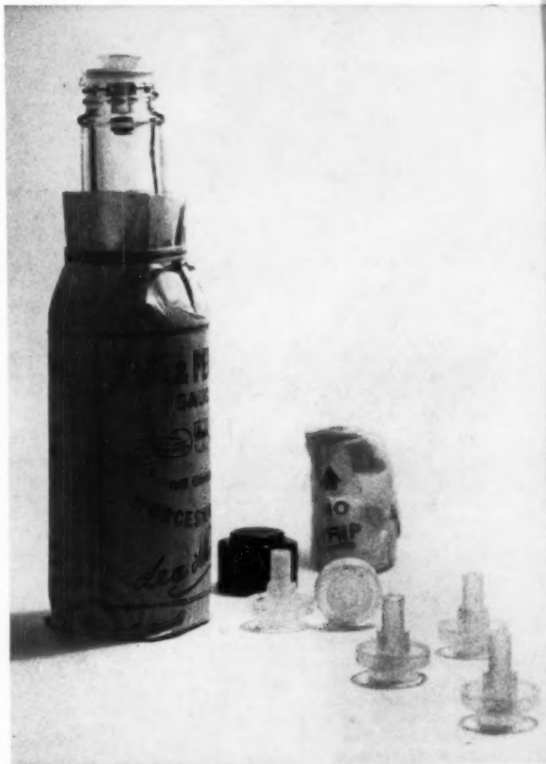
The notched and beveled outer tube and the air pipe control dripping and flowing action. Fitment is made of flexible polyethylene because it is impervious to the product and does not transmit either flavor or odor.
