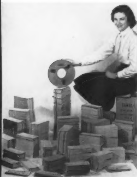
Tape's significance as a miniaturization component is strongly evident in data processing equipment. The reel of magnetic tape shown here is capable of holding the information stored on 28,000 punched cards. In addition to saving space, tape also reduces maintenance.
