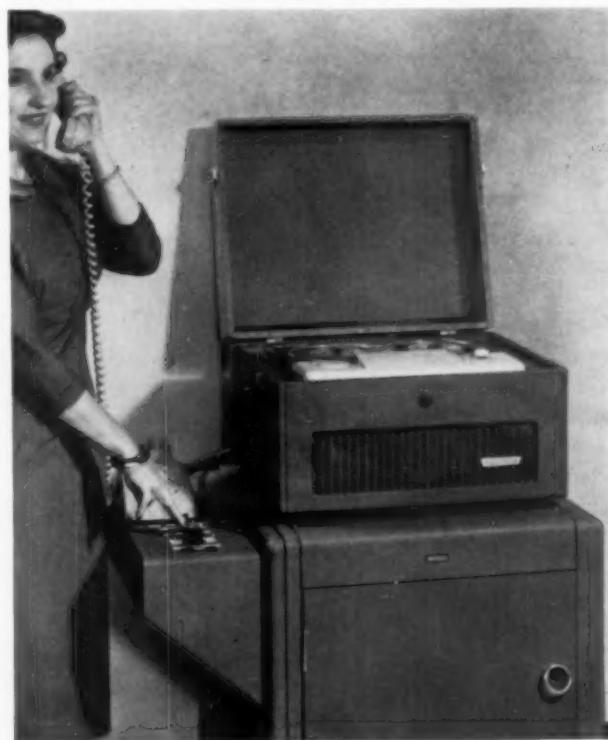
New tape product is Dataphone, below, a system permitting data transmission over telephone lines. Dataphone converts data into tones which are sent over the line, received by another Dataphone which changes the tones back into original messages.
