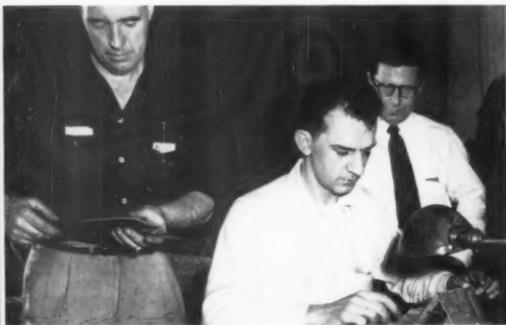
Edge-setting the "900" line. As foreman Gustaf Cyran grinds the final edge, supt. MacQuarrie inspects a finished blade.
