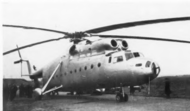
The MI-6, literally a flying boxcar, carries payload of 24,000 pounds at record altitude of 7,874 feet. Designed by Mikhail Mil, it has two turboprop engines, could carry two cars or a bus.
