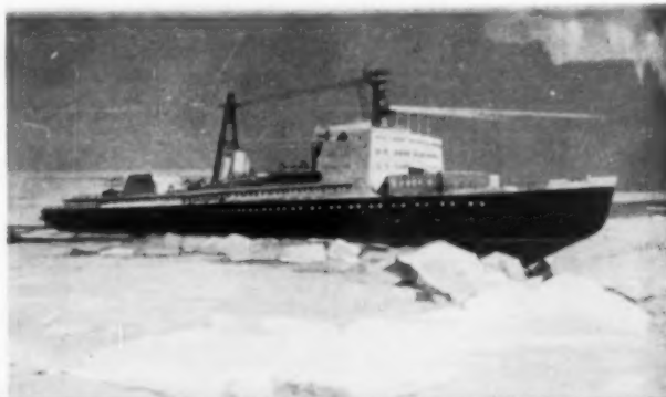
Russia's atomic-powered ice-breaker has a 44,000 horse power engine. The first atomic ice-breaker to be built, it has been shown in model form at the Brussels World Fair and other exhibitions.
