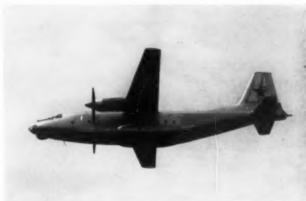
The Flying Whale is a transport ship that carries large machine tools and even small buildings or a city passenger bus. It is fast, can take off and land on very small fields and is quite economical. Oleg Antonov designed the Flying Whale.
