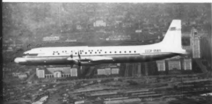
The Moskva, or IL-18 is a four engine turboprop which can handle 12 ton commercial loads at cruising speeds of better than 400 miles an hour. Designed by Sergei Ilyushin, it comes in tourist model, seating 100; passenger, seating 75; and freight.
