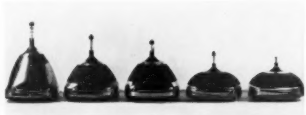
Above: Evolution of picture tubes from early 70° to new 110° points up problems faced by designers in shaping cabinets. Tube at extreme right is Philco's new S-F; next to it is standard 110° tube with longer neck. Below: Portables illustrate progress in tube development, trend towards thinner sets; new 11½" deep model (left) shows how engineering of separate screen sets was applied to produce a more realistic portable. Chassis is fitted around base of tube, with all parts exposed for servicing.
