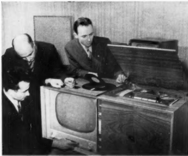
↑ The Temp-5, now being made in the Moscow Radio Factory, includes push-button radio, magnetophone and automatic phonograph. Designers are D. Gendelev, K. Abramyan, and V. Averin.
