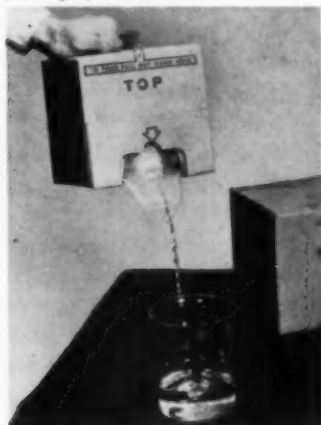
8. Cubitainer pours smoothly since any vacuum caused by liquid discharge is compensated for by folding of container.
