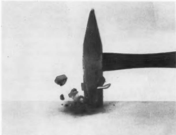
Unsintered parts will fragment when subjected to all but minimal pressures. Die presses powders to final form.
