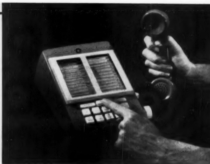
Bell's model of an experimental transistorized telephone instrument (left) uses push-buttons in place of conventional dials; telephone numbers are pre-set in trial telephone instrument (right) and automatically dialed by pushing appropriate button.
