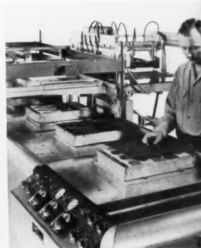
13. Completely automatic skin packaging machine fabricates and splits packages to size.
