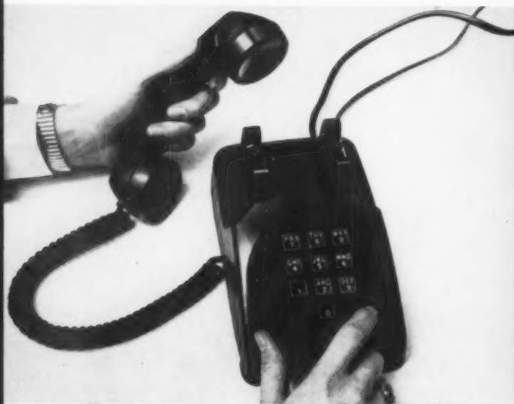
Bell's model of an experimental transistorized telephone instrument (left) uses push-buttons in place of conventional dials; telephone numbers are pre-set in trial telephone instrument (right) and automatically dialed by pushing appropriate button.
