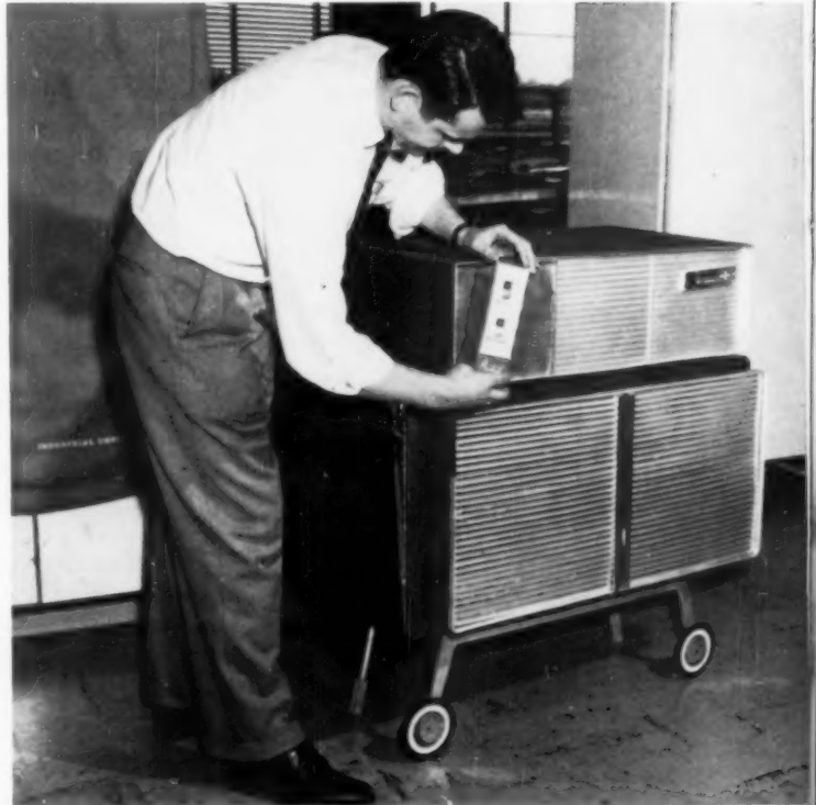
Experiment in thermo-electrics—a hostess cart: refrigerator with oven on top. Acting manager W. H. Appel examines panel.
