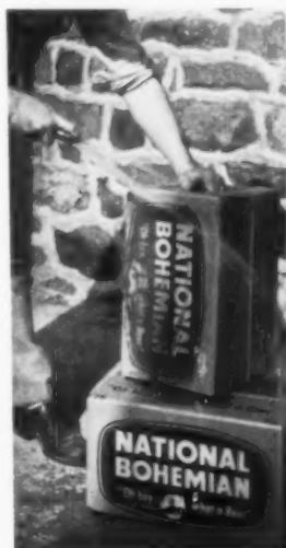
12. Lamination of half mil "Mylar" polyester film makes cartons re-usable.
