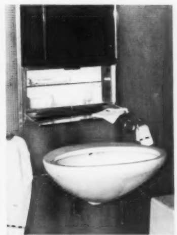
Electronic bathroom (Jules Weydts, Belgium) replaces valves with simple pushbuttons mounted in recessed stainless frame with snap-up front. One button controls temperature of water, which flows into bowl from slits under rim. System operates bathtub by remote control if desired.
