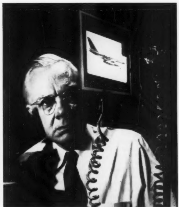
Principle of electroluminescence is used by Sylvania in their Sylvatron (above), an image-producing panel that converts electric data into dots of light; may be forerunner of a flat tv.
