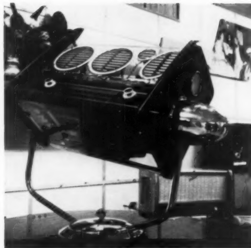
Revolving radio (U.S.S.R.) is mounted in glass case to show mechanism, 3 speaker systems.
