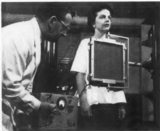
Electroluminescence applied to fluoroscopy results in increased light amplification of image, which means patients are exposed to less radiation. The new amplifier for X-ray viewing (above) is being developed by Radio Corporation of America.
