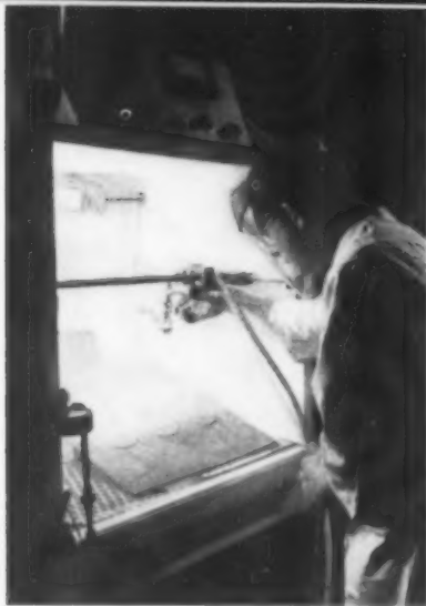
Crux of electroluminescent lamp — phosphor layer — is no knotty problem in production process. At Sylvania's "Panel-scent" lamps production line, layer is applied with spray gun before baking.
