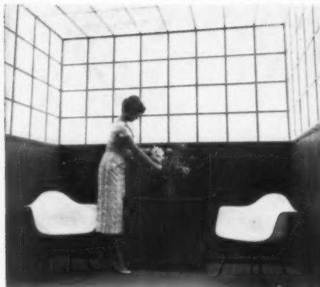
Promise of electroluminescence is seen in this room at Westinghouse Research Labs; parts of walls and ceiling consist of the new glowing panels no thicker than window glass. Home installation of new light is not yet economically feasible.
