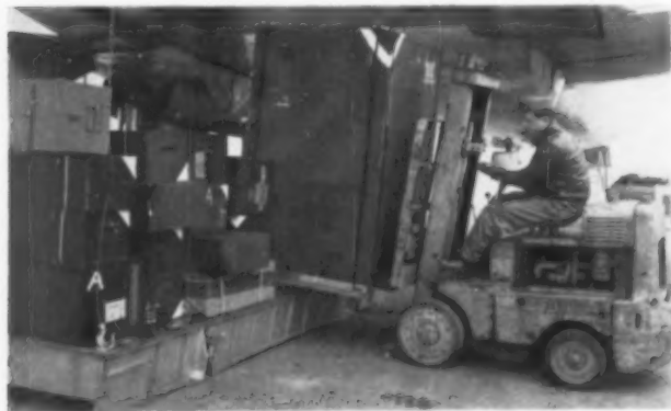
The fork-lift truck moves modular containers to loading platform of waiting air transport. The modular container system was Becker & Becker's first assignment for the Air Force. Each case opens out to be a piece of ground support equipment. The difference in bulk and ease of moving can be judged by comparing modular units with hodge-podge of old-fashioned crates at left.
