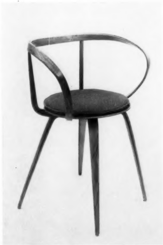
↑ George Nelson's "pretzel" chair shows some of the problems of designing for laminated wood—multiple bends, for instance, and varying thicknesses. These are solved by special woodworking techniques: the arm-and-back strip gets a Moebius-strip twist; laminations of different lengths are compiled to achieve tapered shape. From Herman Miller. Chair, with cushion, lists at $116.
