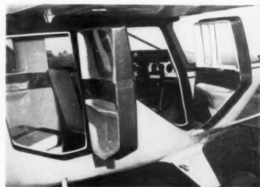
Doors of the Taylorcraft model are also made of the reinforced material. Each door consists of two moldings, the outside frame, and the inner lining. The armrest is part of the inner lining; single mold fits inside frame, facilitates assembly.
