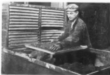
Drying tray for corrosive chemical intermediate is molded of American Cyanamid's Laminac polyester and glass fibers.
