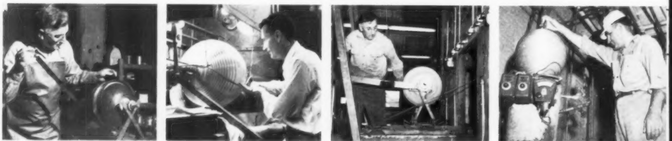
Filament winding of reinforced plastic pressure bottle at Apex Reinforced Plastics Div., White Sewing Machine Corp., Cleveland, starts with covering basic form with rubber gaskets (extreme left). Sealed, the rubber mounting forms interior of bottle. Resin-impregnated fibers are then wound on form (second from left) by pendulum type needle arm. Next, the sphere is placed in an oven, and basic form is melted out (extreme right) before bottle is finished, tested, and shipped.
