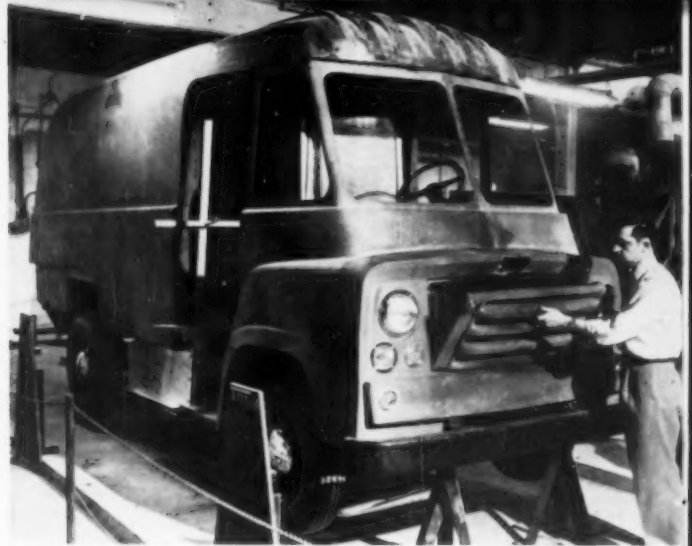
All-plastic body of United Parcel Service delivery truck is made up of 22 parts molded separately by the vacuum bag technique. Use of plastic meant 60% saving in weight. Manufactured by Lunn Laminates, Inc., Huntington, N. Y.
