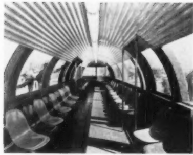
Steel-ribbed frame of the monorail coach above, in operation in Houston, Texas, is covered with reinforced plastic. The shell was constructed in sections by Consolidated General Products.
