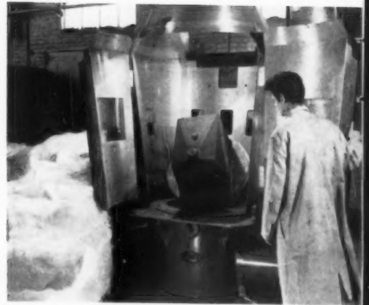
The plenum chamber method for forming the reinforcement is shown above. Here the fibers are deposited on the screen automatically. Fed from the top, the cut fibers are drawn onto the screen by a vacuum below it.
