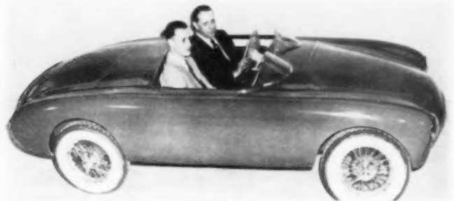
Chassis and underbody of Renault's sports car "The Rogue," were molded separately, then assembled. Celanese Marco Resins were used exclusively for the lightweight, weather resistant body. One of the early all plastic body cars.
