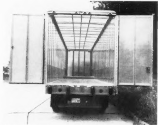
Panel construction is used in this trailer body for the Celanese Corporation. Translucent panel makes it possible to read large type on packing cases stowed against inner sides of van. Made of reinforced Celanese polyester by Alsynite Company of America.
