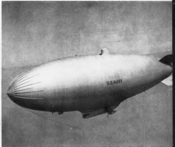
Navy blimps bristling with reinforced plastic radomes are another link in the defense system. These domes are strong, do not interfere with high frequency waves, yet are light enough for blimps.
