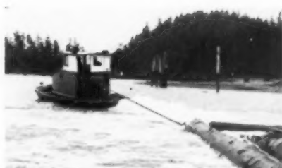
Fiber glass-reinforced hull of 28-foot tugboat above, permits craft to lie on mud flats at low tide; solvent-resistant properties of material prevent damage. Molders: Skagit Plastics, Inc., La Conner, Wash.
