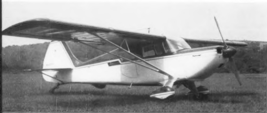
Wings as well as body of Taylorcraft are a product of reinforced plastics. Made by Taylorcraft Inc., Conway, Pennsylvania. Richard Arbit, designer.
