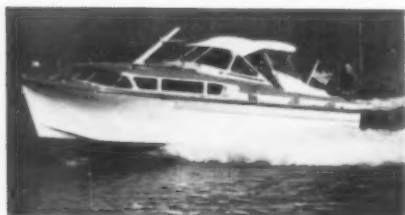
Large, 31-foot stock cruiser at left illustrates the full extent of reinforced plastic use in boat construction. Not only the body but refrigerator, tanks and sink are made of fiber glass-reinforced plastic. Boat built by Skagit Plastics, Inc.
