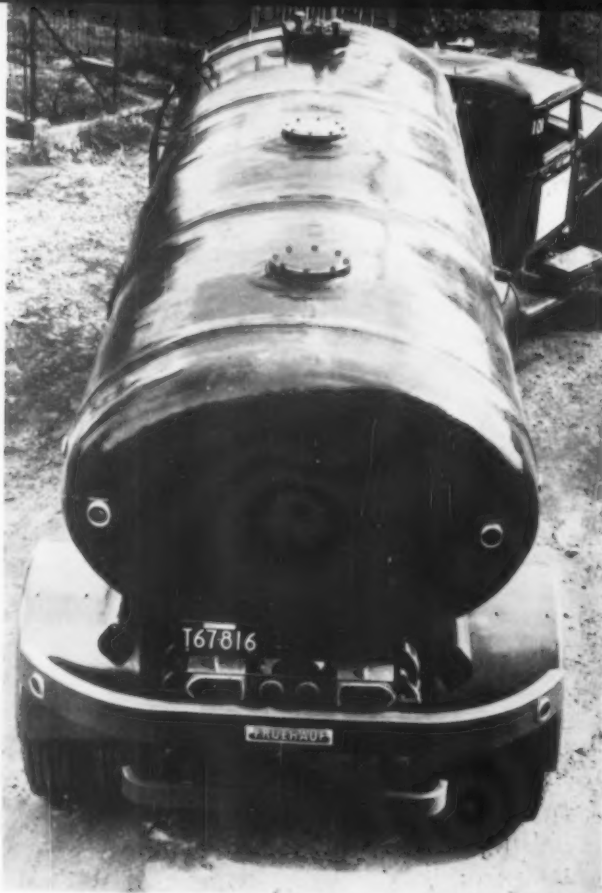
Large fuel carrying tanks are made of fiber glass saturated with American Cyanamid Laminac resin. In addition to chemical resistance, reinforced plastic tanks have 1/3 more capacity than steel tanks of equal weight.
