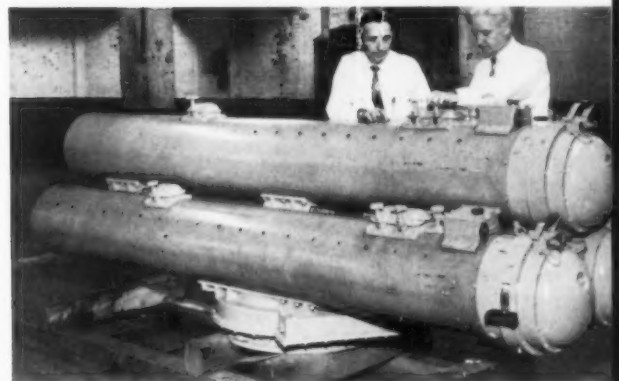
An offshoot of filament winding, and similar to it, is the centrifugal molding process. It assures uniform wall thickness and eliminates all seams. Above, torpedo tube housing molded by Apex Reinforced Plastics. Similar shapes like hot water tanks can be centrifugally molded.
