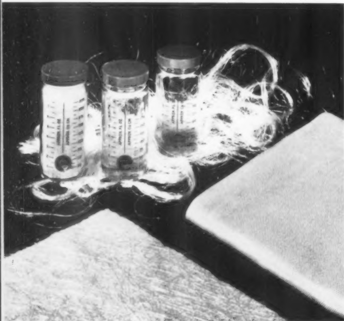
Three basic types of glass reinforcements are shown above. Continuous strands, known as rovings, are cut for use in the preform process. Reinforcing mats (left) are made of chopped strands with a resin binder. Woven fiber glass cloths (right) provide very high strength; are made in many thicknesses and weaves.
