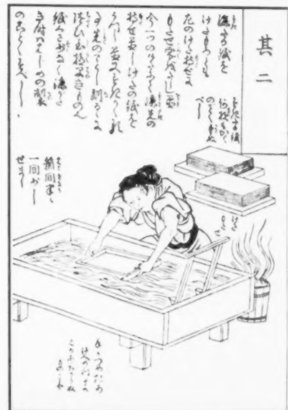
A woman forming Hanshi paper, dipping mold into vat. In background are neat piles of newly-formed stock. The paper is then dried and packed. The text says woman complains of the coldness of her hand.
