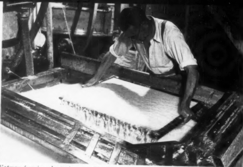
Vatman forming sheet of paper. The surplus pulp runs over far side of mold. Mold is of light construction because weight of pulp and suction is great, as can be seen by tensesness in muscles. Experienced vatman forms many sheets, all "uncannily" of same weight.
