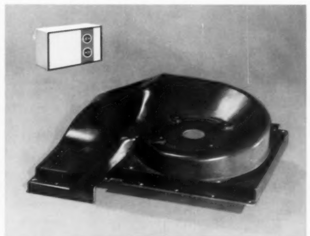
AIR-CONDITIONER PARTITION MOLDED OF PRE-MIX POLYESTER. Pre-Mix can be molded in varying contours of an Archimedes spiral—all in one piece construction. Partition is corrosion-proof and acts as a thermal barrier.
