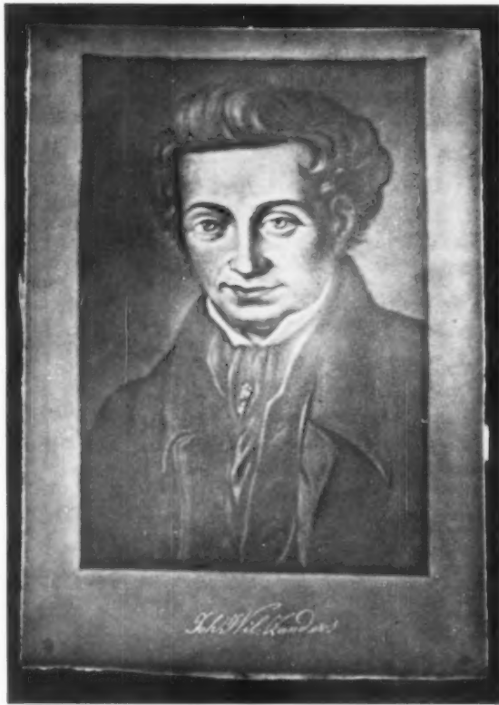
Five hundred years after the invention of line watermarks came "chiaroscuro." These remarkable sheets of paper show this watermarking technique carried to its highest degree of perfection. On the left, a portrait from the J. W. Zanders (Bergisch Gladbach, Germany) collection, and on the right, a view of St. Peter's in Rome. Latter is from the mill of E. Miliani of Fabriano, Italy. Wm. H. Smith, an Englishman, invented this process of embossing a bas-relief on a wave covering. The Zanders watermark measures 8" x 11½", the Fabriano, 14½" x 17½". Use of this kind of watermark is sadly unexploited today as a part of letterhead design.
