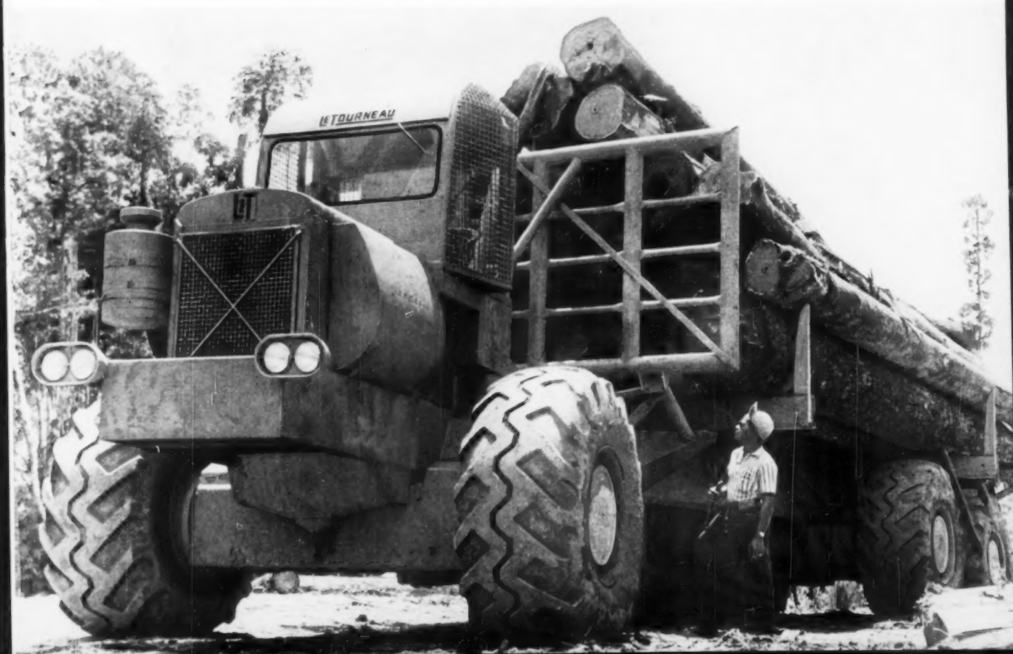
The Electric Logging Arch (above) skids up to 28 tons of heavy timber along even rough jungle trails. Tires with deep-cut treads churn through mud, easily negotiate the steep grades and sharp turns.
