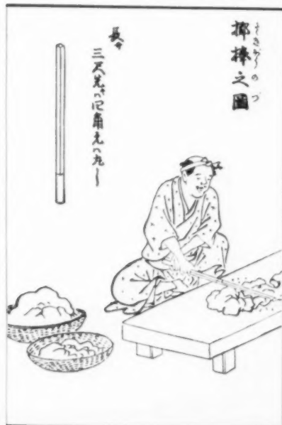
The papermaking bark is shown here being beaten. (A typical beating stick can be seen at upper left-hand corner.) This work, which is near the end of the process, takes much time and patience to perform.
