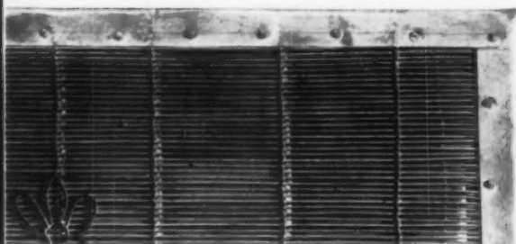
A corner of a "laid" mold showing copper stripping holding down complex of wires. It is this criss-cross of "laid" and "chain" lines that makes ribbed appearance.
