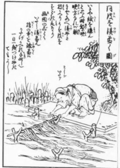
The bark is then immersed in a running stream for a period of time in order to remove all imperfections, such as knots. The Japanese call the product at this stage of the process Siro-Kawa (white bark).
