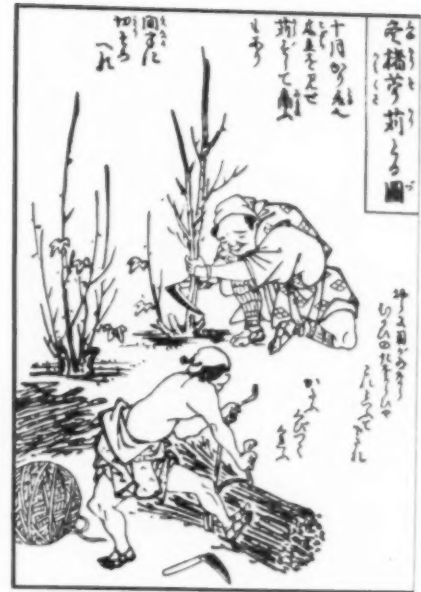
The first step in papermaking process is getting the raw material. Here branches of plants suitable for paper are being cut evenly in middle, cinched tightly in large bundles and are then sold to papermakers.
