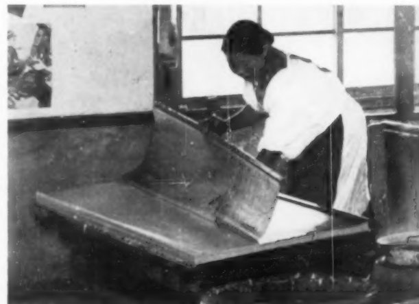
A Japanese papermaker removing wet sheet from flexible bamboo mold covering. The wet sheet is simply pulled off the covering and neatly stacked. Use of Tororo-aoi mucilage prevents sticking.
