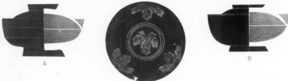
Two forms of traditional Kashiwa-Mon bowl; thinner wall, shallow base, flared rim of the right-hand bowl are functional adaptations.
