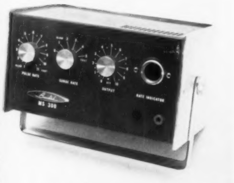
234 Muscle stimulator The Burdick Corporation, Milton, Wisconsin Don Doman Associates, consultants 1/8" brake-formed aluminum wrap serves as chassis and housing. Edges are polished, sides painted. Handle can serve as stand.
