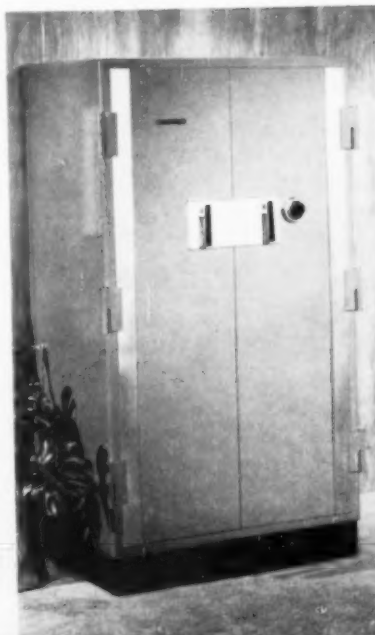
147 Fire-insulated safe Meilink Steel Safe Co., Toledo Ralph E. McClellan, design engineer Sundberg-Ferar, Inc., consultants Expansion joint and pre-stressed stay rod construction; thermo-cel insulation solid cast and encased between inner and outer shells.
