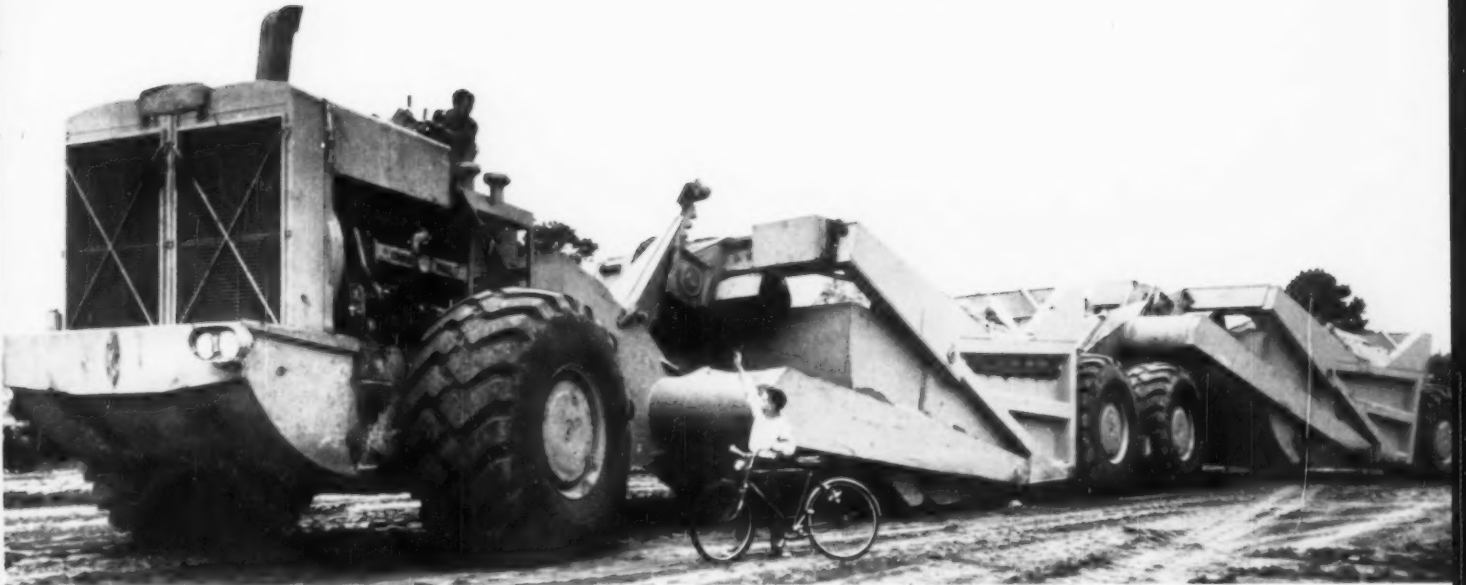
211 Super earthmover R. G. LeTourneau, Inc., Longview, Tex. Staff design Two giant buckets are incorporated in the self-loading earthmover to hold the 130 ton load. Newest and biggest of all earthmovers.
