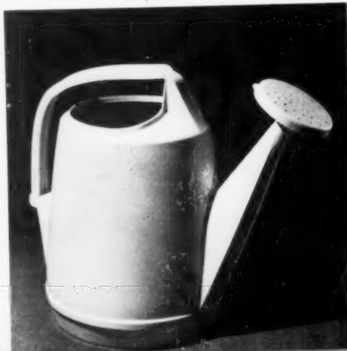
105 Sprinkling can Federal Tool Corporation, Chicago John E. Press, Chief Engineer Reinecke & Assoc. (Jack Mell), consultants Polyethelene bucket and handle molded in one piece; handle end snaps onto rim.
