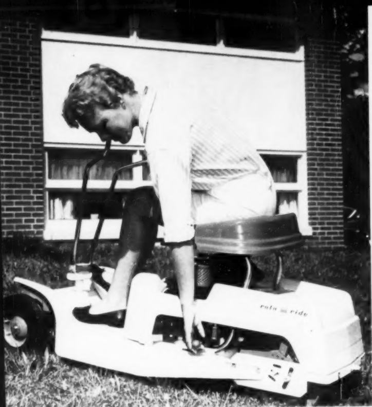
122 Power lawnmower Moto-Mower, Richmond, Indiana Blade of riding mower stops instantly when lock-out lever is thrown.
