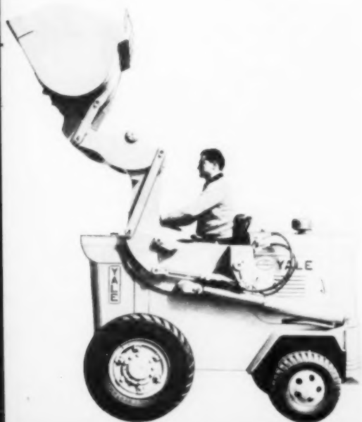
212 Tractor shovel Yale & Towne Manufacturing Co., New York Staff design Rear end casting employed to provide a counterweight and sturdy grille to protect the radiator and headlights.
