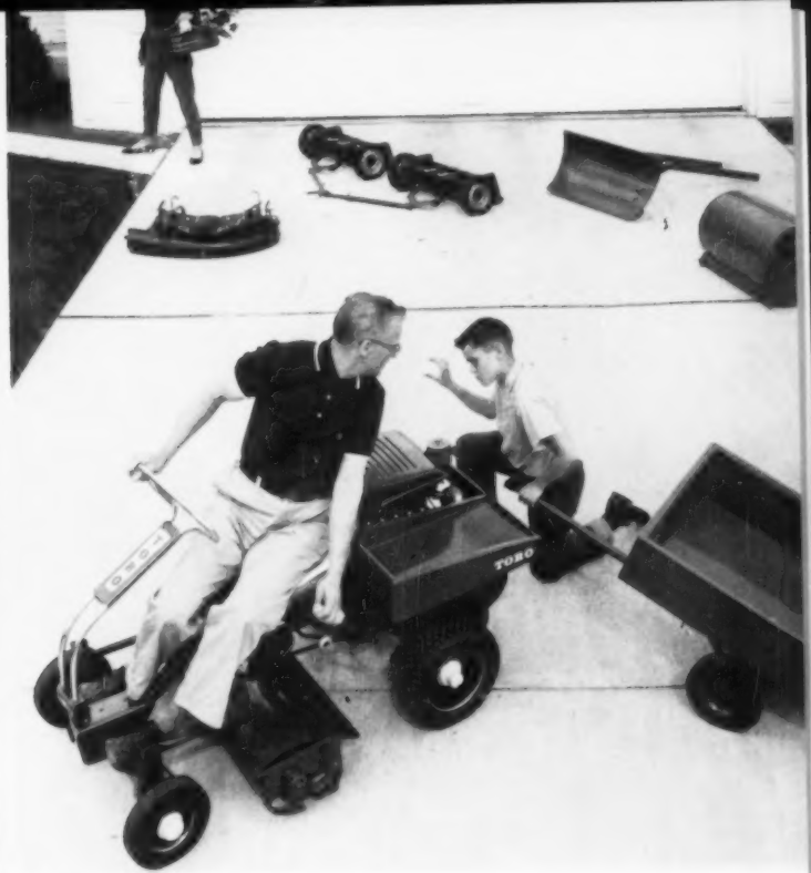
123 Garden tractor Toro Manufacturing Company, Minneapolis Staff design Charles Butler, consultant Sportsman model, 5.75 h.p., bevel gear transmission. Steering bar swivels for access to seat.
