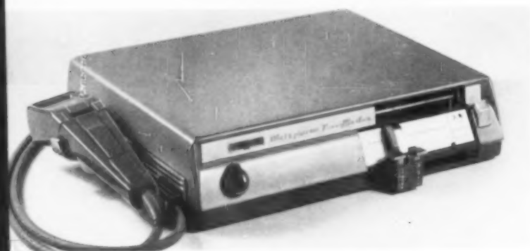
143 Dictating machine Dictaphone Corp., New York Gordon Florian, designer Extensive use of aluminum for mechanical components, magnesium case, transistorized amplifier effect 20% weight reduction.
