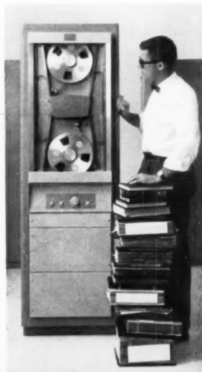
128 FR-300 hi-speed digital tape transport Ampex, Redwood City, California Staff design Frank T. Walsh, designer Complete equipment fits one 19" rack cabinet, tape speed of 150 ips; 10 1/2" reels; 1/2" or 1" tape.
