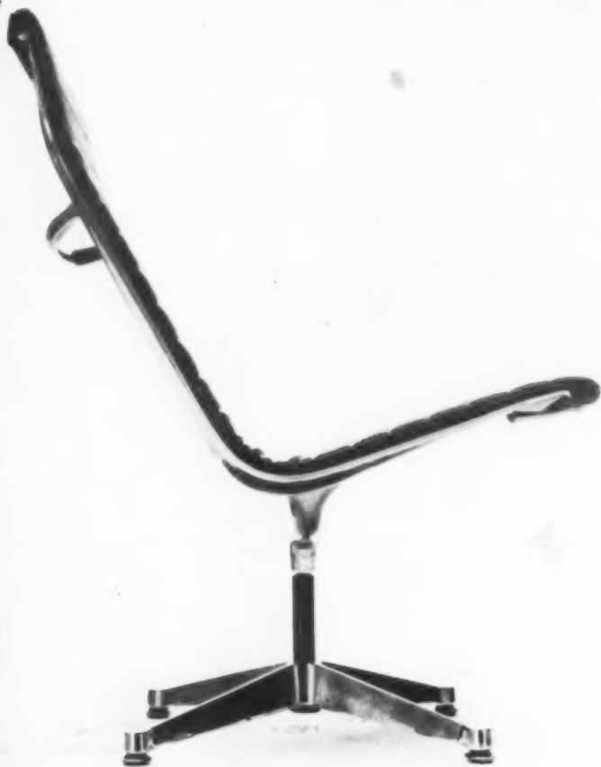
12 Chair Herman Miller Furniture Co., Zeeland, Mich. Charles Eames, designer Side frames and stretchers of grooved aluminum castings. Electronically welded Naugahyde upholstery—reinforced by stiff inserts—is held in tension. Swivel base.
