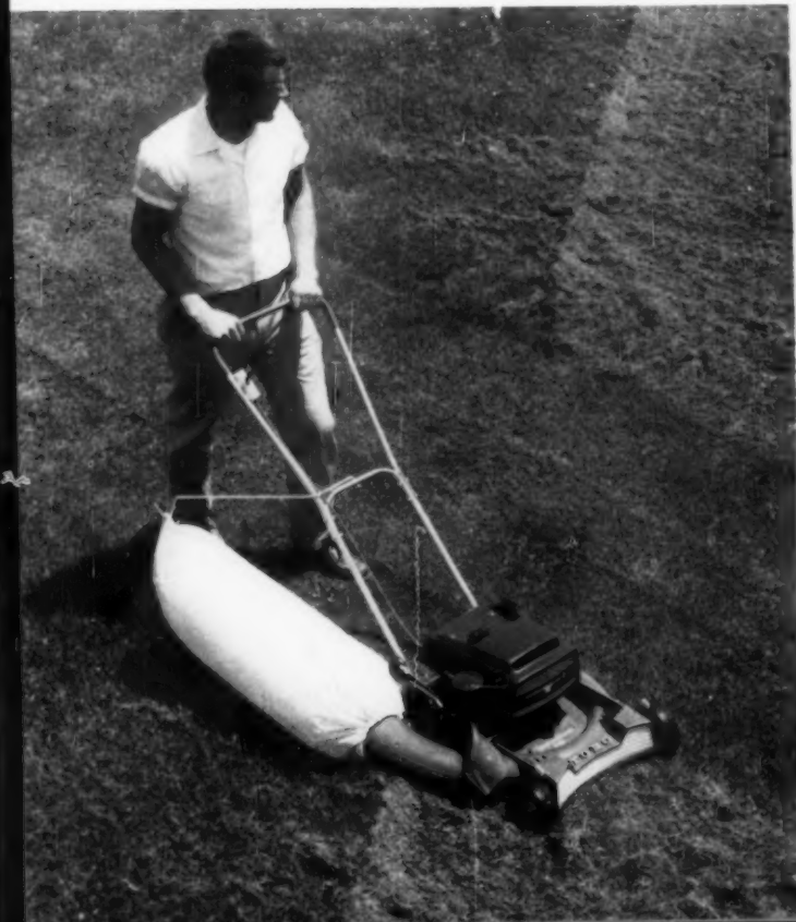
124 Power lawnmower Toro Manufacturing Company, Minneapolis Vacuum forces blades upright for cutting; air flow forces cut grass into bagging attachment. Leaf mulcher included.
