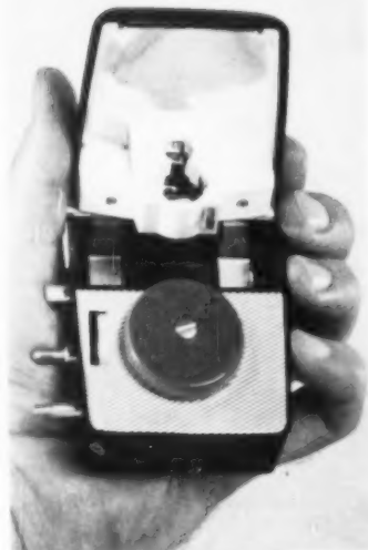
166 Kodak Generator Flashholder Eastman Kodak Company, Rochester, N. Y. Staff design No batteries needed. Half-turn of nylon generator wheel stores electricity in capacitor to fire M-2, No. 5, or new M-5 or M-25 flash bulbs.
