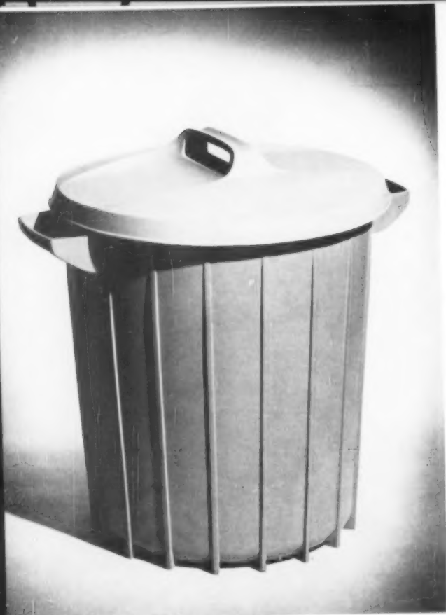
102 Refuse container Rubbermaid, Inc., Wooster, Ohio Clyde Breneman, staff designer Smith, Scherr & McDermott, consultants Molded of polyethelene; structural ribs act also as feet. Lid locks on.
