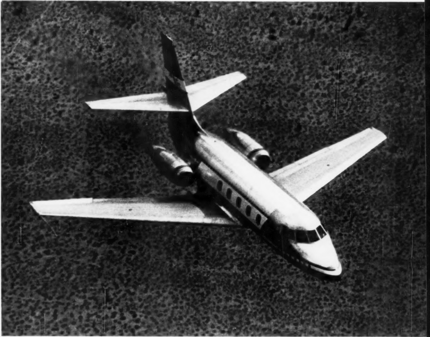
229 "Jetstar" Lockheed Aircraft Corporation, Burbank, Cal. Staff design Kelly Johnson, chief designer Top speed 685 mph; has flown at altitudes of 32,000 feet, and non-stop 3105 miles.
