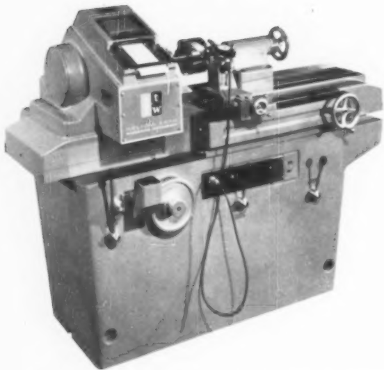
231 Helical Lead Measuring Instrument Illinois Tool Works, Chicago, Illinois Re necke and Associates, designers Measuring instrument keeps record of each gear, which is checked on tape.
