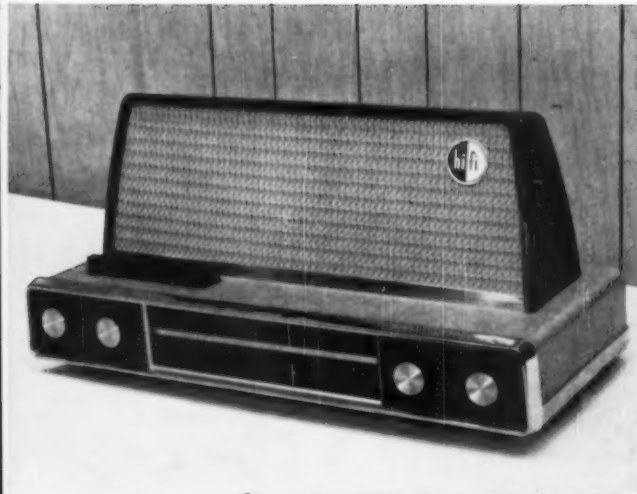
† Arvin 3586. James F. Mariol, designer. Vinyl-laminated steel cabinet; cloth grille; 10 tubes, 2 speakers; phonograph jack. $100.
