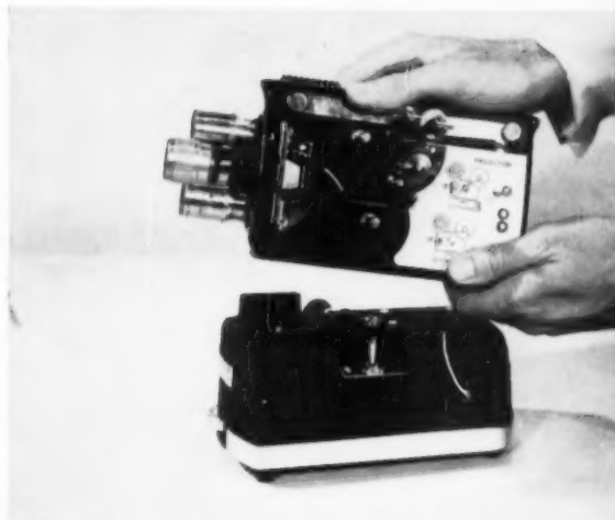
Wittnauer 8 mm Cine-Twin. 400-watt, camera-projector. 3 taking lenses (standard, wide-angle, telephoto), 1 projection lens and zoom finder. Reel-holding arms fold out from top, which is then placed on base containing motor, cooling system, controls. Front reel arm, when raised, opens passage for projection light.
