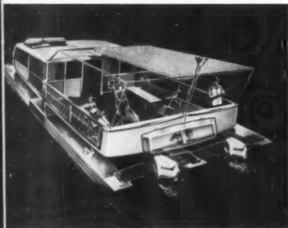
Brook Stevens designed the "Housefloat" (left) for Evinrude. The fiber glass and aluminum boat, expandable because of its modular construction, is indicative of the quite different direction of Evinrude's promotion. Such futuristic styling is intended to stimulate outboard boat manufacturers to design their boats to keep pace with the latest developments in outboard motor design by incorporating many of the basic marine features of these boats of the future.
