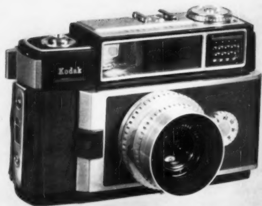
Kodak Signet 80 with 50mm f/2.8 Kodak Ektanar rare-element lens. Has both Light Value Scale and f / value. Built-in photo-electric exposure meter measures both incident and reflected light in LVS and shares "control tower" with viewfinder and rangefinder. Includes parallax correction. Styled in black and satin metal.
