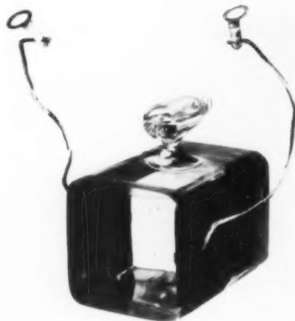
Avco's Kerr Cell is filled with nitrobenzene, has pair of flat electrodes with optically clear "windows" at both ends and Polaroid filters over both windows. This electro-optical shutter and pulse generator circuit (complete shutter package measures 12x12x5") achieves exposure time of a hundred-millionth of a second.
