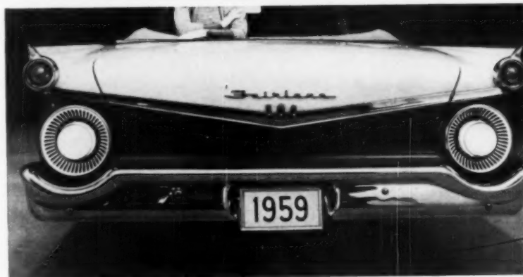
Bright reflectors circling Ford's big tail lights make them seem even bigger. Back-up lights have been positioned high into rocket-like fins. Low coaming on Ford's big trunk makes access easy.
