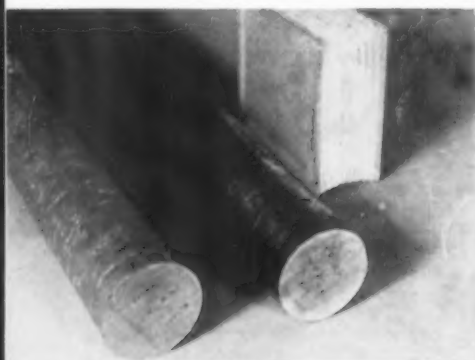
Columbium must be protected against contamination, and is expensive as a result. Mill shapes can be rolled or drawn, and cost approximately $90 per pound.
