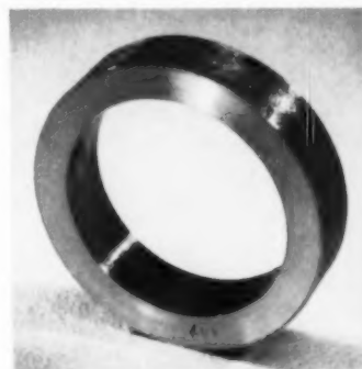
One of important metals of atomic age is zirconium. Zirconium tubes (cross-section shown here) are used in reactors.
