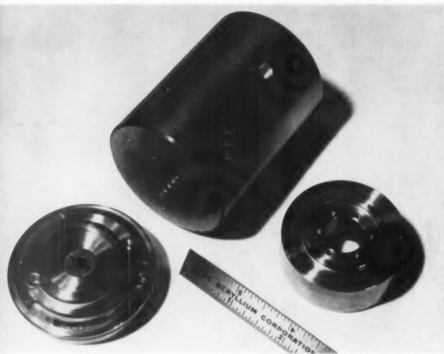
Beryllium bar and rod stock can be fabricated by extrusion and can be machined like the pieces (at left) produced by the Beryllium Corporation. While machining, extreme cleanliness is one of a great many precautions which must be taken.
