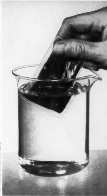
Putnam brand fabric dyes are packaged in water-soluble polyvinyl alcohol film designed to do disappearing act when dropped in cold water. Picture at left shows pouch being immersed. At right, a few minutes later, pouch is stirred into nothingness.
