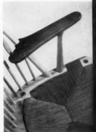
Legs, arm, and back of armchair interlock in intricate joinery; arms of Windsor chair lap around rods of back.
