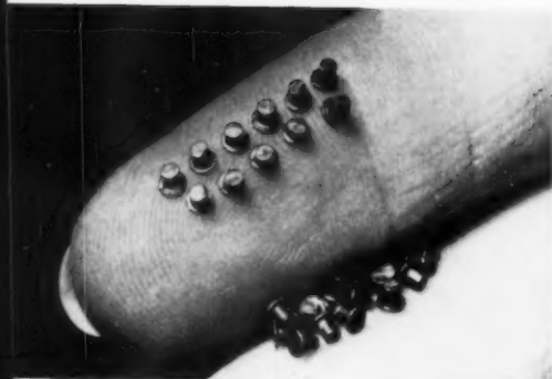
The molybdenum rivets at left were produced by Westinghouse from molybdenum wire, and are applied where high temperature resistance and strength are important material requirements (in electron tubes or molybdenum radiation shield furnaces).
